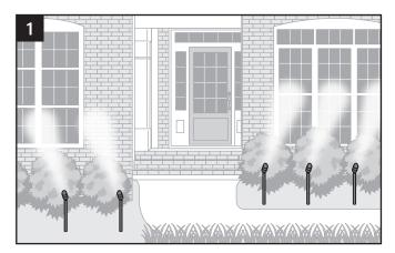
1. Locate placement of spotlights and lead wiring. Plan accordingly if you choose to bury wire under concrete or other permanent structures. 2. Connect male lead from light to female to one end of female adaptor.
