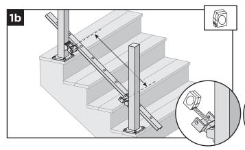
1b. With brackets in correct swivel locations, measure distance from inside of swivel bracket to inside of swivel bracket. Ensure that before cutting, balusters holes are parallel and centered in between the posts and also allow for clearance for attachment to brackets. Mark bottom stair rail at each intersection.
