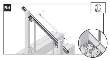
5d. Position top rail onto balusters (position to side of post) and ENSURE that balusters are parallel with post. With brackets in correct swivel location, measure distance from inside of swivel bracket to inside of swivel bracket. Mark top stair rail at each intersection.
