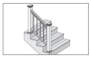
**Important: ONLY** use for use with pressure treated 4 x 4 post (3.5" nominal square) and 4" x 4" (102 mm x 102 mm) or 6" x 6" post sleeve. Trex Signature Posts, Trex Post Mounts or Joist Mount Posts cannot be used with Signature Traditional railing.
