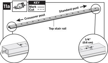
11a. Top stair rail along with rail insert must be cut differently on each side of the rail. Railing side that attaches to standard post should be cut 1/4" (0.6 cm) shorter than the mark to allow for fit into top rail bracket. Railing side that attaches to the crossover post should be cut directly on the mark to allow for fit into the crossover post bracket.
