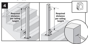
4. Measure up required dimension for 36" (91.4 cm) tall railing or 42" (106.7 cm) tall railing, from top of lower stair rail fixed bracket. Mark with light line.
