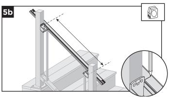
5b. Position top rail onto balusters (position to side of post) and ENSURE that balusters are parallel with post. Mark top stair rail at each intersection.
