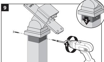
Attach stair crossover swivel bracket to post with two self-tapping screws (provided). Slide cover over post to hide screws.
