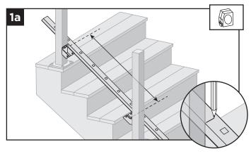
1a. Position bottom stair rail along the nose of the stair treads. Ensure that before cutting, balusters holes are centered in between the posts and also allow for clearance for attachment to brackets. Mark bottom stair rail at each intersection.
