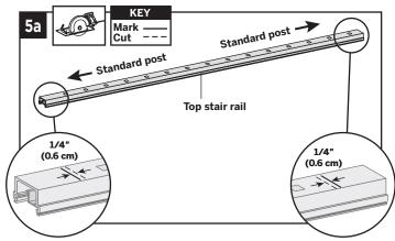
5a Cut each end of top stair rail along with rail insert 1/4" (0.6 cm) shorter than mark to allow for fit into
