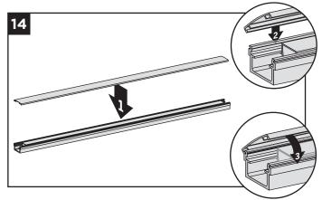
14. Attach "crowned" upper stair rail cover to upper stair rail by aligning cover on one side of rail. Then starting from one end of stair rail, snap cover onto opposing slot working down length of stair rail. A **rubber mallet** may facilitate the fastening using **GENTLE** tapping.
