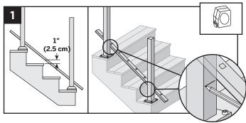
1. Lay bottom stair rail on steps beside posts. Position bottom rail at least 1" (2.5 cm) **above** nose of stair tread.
