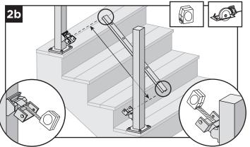
2b. Cut each end of the bottom rail, rail insert, and bottom rail cover at the mark on each end to allow for fit into bottom stair rail brackets.
