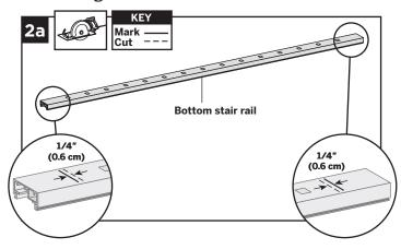
2a. Cut each end of the bottom stair rail, rail insert, and bottom rail cover 1/4" (0.6 cm) shorter than the mark on each end to allow for fit into bottom stair rail brackets.
