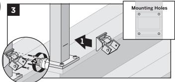
3. Center lower stair swivel bracket on post above the marked line and attach using four self-tapping screws (provided). In some cases it may be difficult to attach the stair bracket on the lower stair post. Recommend using a 90° cordless drill in this area if possible to attach screws.
