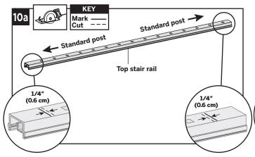
10a. Cut each end of top stair rail along with rail insert 1/4" (0.6 cm) shorter than mark to allow for fit into top stair rail bracket.
