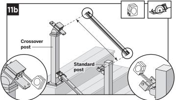
11b. When going from standard stair post to stair crossover post, measurement must be taken from inside of top horizontal stair swivel bracket to inside lip of stair crossover bracket (crossover post will need to be modified to have swivel crossover bracket installed).
