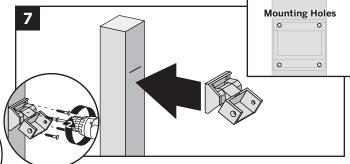
Center upper stair swivel bracket on post **below**the marked line and attach using four self-tapping
