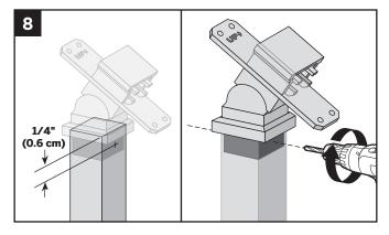
8. Once location/height is determined, center and predrill two holes (using a drill bit slightly smaller than that of self-tapping screw diameter) on opposite sides of post, approx. 1/4" from top of post. Drill through the post and into the stair crossover swivel bracket on each side.
