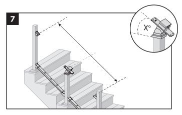
7. Determine location/height of the stair crossover swivel bracket by aligning the angle of this with the fixed brackets (or compound swivel brackets) already installed.
