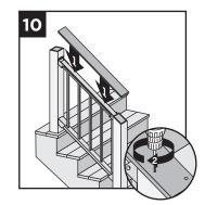
BOARD MAY REQUIRE EITHER A NOTCH CUT ON THE UNDERSIDE OR SLIGHT PLANING ON THE UNDERSIDE TO ALLOW DECK BOARD TO CLEAR TOPS OF BRACKETS AND SIT FLUSH ON TOP OF POSTS AND RAILS. Attach boards on each post with Trex-recommended composite screws (quantity of 2 per each board end).
