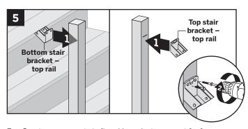
5. Center upper stair fixed bracket on post **below** the marked line and attach using two self-tapping screws (*provided*).
