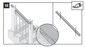
18. Place 2" x 4" (51 mm x 102 mm) beside top rail. Mark and cut (both ends need to be cut on an angle for proper fit).
