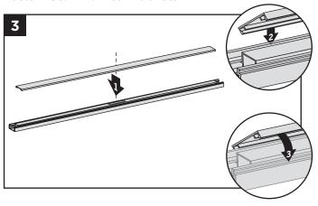
3. Attach "flat" bottom stair rail cover to bottom stair rail. Align cover on one side of the bottom rail in slot on side of rail. Then starting from one end of rail snap cover onto opposing slot working down the length of the rail. In some cases, a **rubber mallet** may facilitate the fastening using **GENTLE** tapping.
