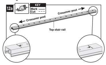
12a. Cut each end of the top stair rail along with rail insert on the mark line to allow for fit into the crossover post bracket on each side.
