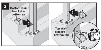
2. Center lower stair bracket on post above the marked line and attach using two self-tapping screws (provided). In some cases it may be difficult to attach the stair bracket on the lower stair post. Recommend using a 90° cordless drill in this area if possible to attach screws.
