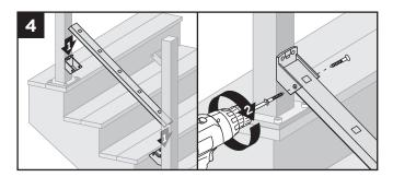
4. Set bottom stair rail into bottom stair rail brackets. Attach bottom stair rail to bottom stair bracket using two self-tapping screws (provided) on each side of bracket.
