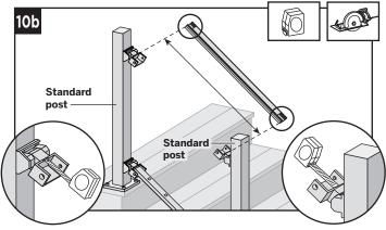
10b. Cut top rail along with rail insert to the measurement between the top stair swivel brackets. For standard post to standard post configurations this would be same dimensions as that of the bottom stair rail.
