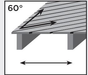
At a 60° angle, maximum joist spanning is 2" (51 mm) less than listed in the chart below.
