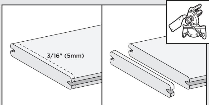
**It is recommended that boards be clean cut on both ends a minimum of 3/16" (5mm).**
