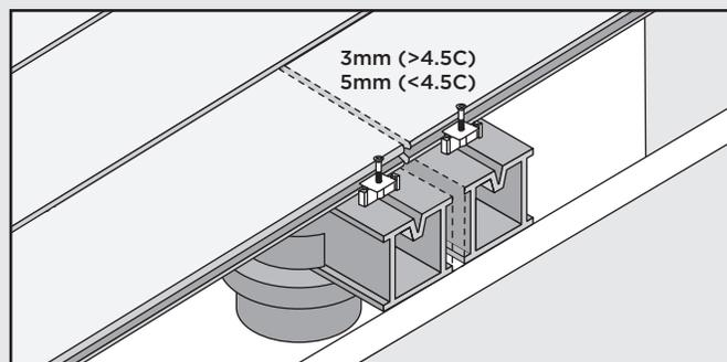
**NOTE:** Hidden Fasteners MUST be used at every joist.
