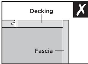
Install fascia **UNDER** decking edges/ends. This will provide protection to the fascia/framing seam as well as optimize the aesthetics of the installation.
