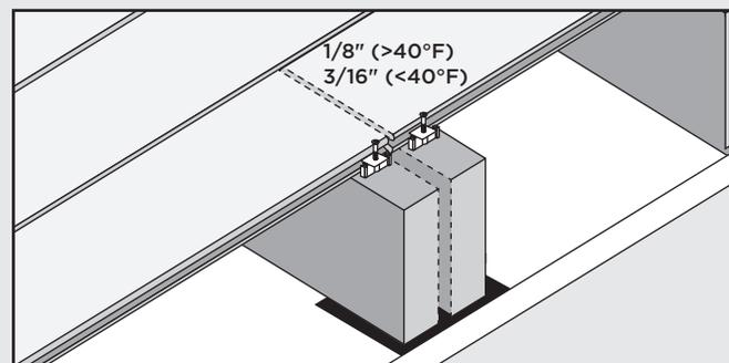
**NOTE:** Optional - Gap joist framing 1/8" - 1/4" to allow for water drainage.
