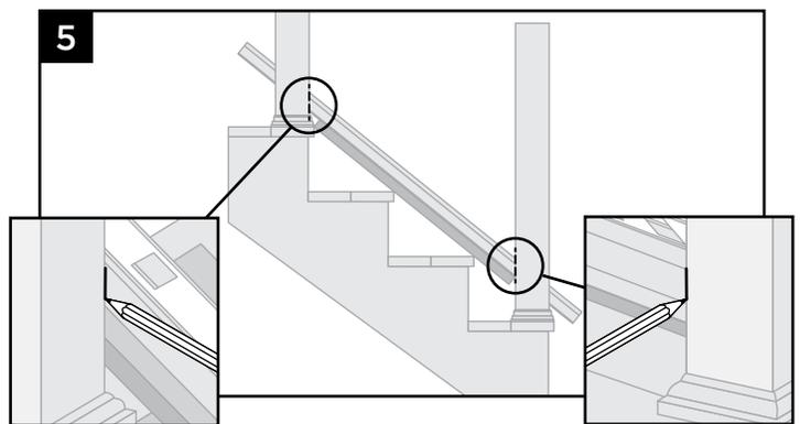
5. Use the lower and upper stair post to set the length of the bottom stair rail. Ensure that baluster spacer holes are spaced evenly between posts. Also allow for a minimum of 1-1/2" (292 mm) at each end of the stair rail for bracket placement and baluster clearance. Mark rail at post intersections.
