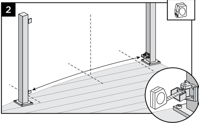
2. With brackets in correct swivel location, measure distance from inside of bracket to inside of bracket. **BEFORE CUTTING, ENSURE THAT BALUSTER HOLES ON BOTH BOTTOM AND TOP RAIL LINE UP.**
