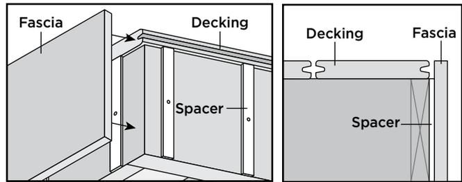
Install 3/16" to 1/4" thick x minimum 1" wide exterior grade spacers (these should be cut the same length as the rim joist), and spaced 9" on center. Install fascia screws as stated below at spacer locations (ensure that spacer screw does not interfere with fascia screw).
