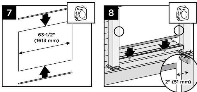
7. Push black edge trim onto top and bottom edges of glass panel. Be sure trim runs entire length of glass. Extra trim can be cut with razor blade or scissors.
