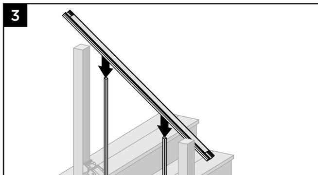
3. Position top stair rail onto balusters ensuring balusters are fully seated in top rail (position to side of post) and **ENSURE** that balusters are parallel with post.
