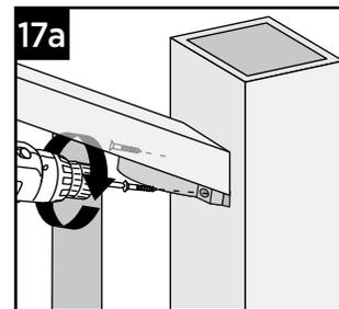
17a. Attach top stair rail bracket to upper post using two #8-10 x 3" screws (provided).
