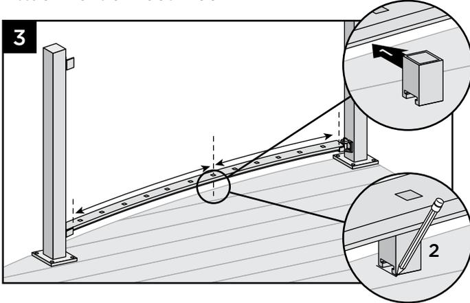
3. Temporarily set bottom rail into bottom brackets, and place Foot Block under bottom rail centered between bottom brackets. Mark to provide placement location of base. Remove bottom rail.
