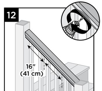
**NOTE:** Balusters can be shifted out of the way if necessary.
