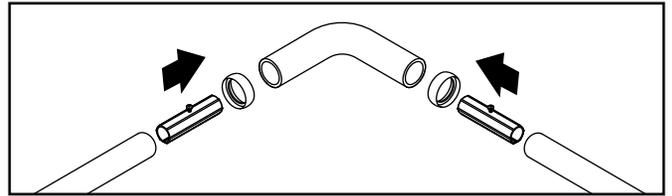
1. If required, cut railing to proper length based on location of elbows and other components being used.
