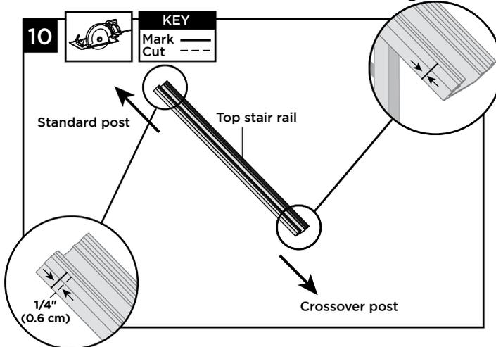
10. Top stair rail must be cut differently on each side of the rail. Railing side that attaches to standard post should be cut 1/4" (0.6 cm) shorter than the mark to allow for fit into top rail bracket. Railing side that attaches to the crossover post should be cut directly on the mark to allow for fit into the crossover post bracket.
