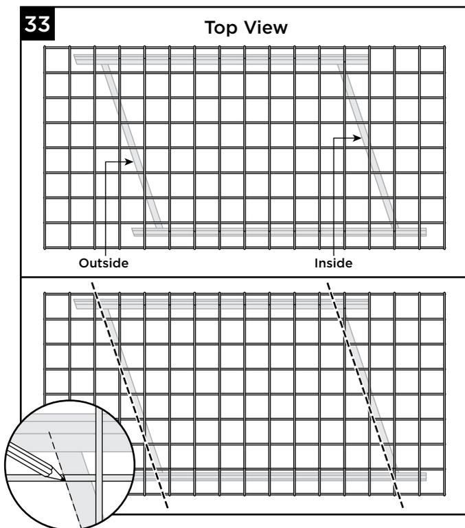
33. For the vertical measurements, align straight edge with **OUTSIDE** of one vertical and mark mesh at all intersection points. Align straight edge with **INSIDE** of opposite vertical and mark mesh at all intersection points.
