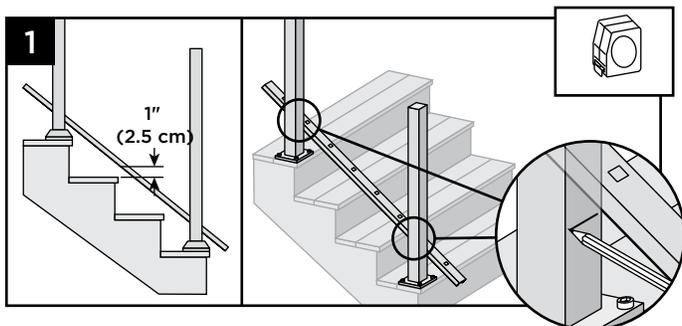
1. Lay bottom stair rail on steps beside posts. **Position bottom rail at least 1" (2.5 cm) above nose of stair tread.**
