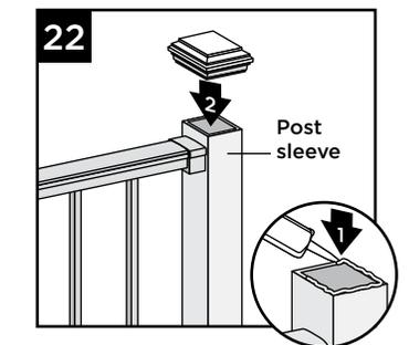
22. Attach post caps to post sleeves using external grade PVC construction adhesive (apply adhesive on the inside self-centering/corner tabs).
