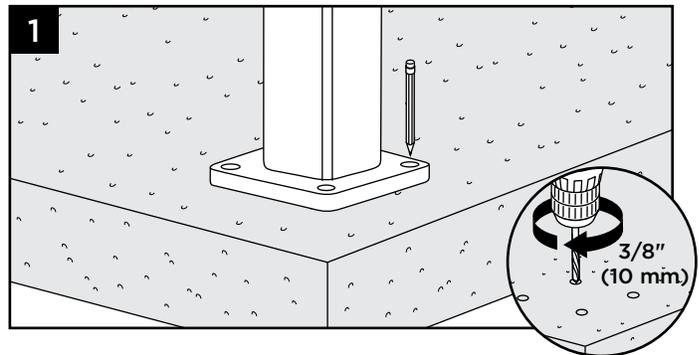
1. Using post as a template, mark locations of the four holes and drill into concrete at least 2-5/8" (66.7 mm) using a 3/8" (10 mm) masonry bit.
