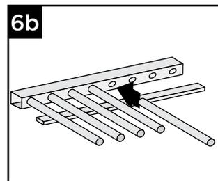
6a. On a clean flat surface, lay bottom railing on its side. Make sure to allow enough room for installation of balusters and top rail. Place a scrap piece of 1" (25 mm) decking board running parallel to bottom rail for support when installing balusters.
