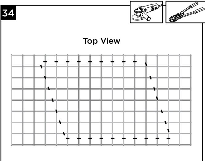
34. Cut mesh at all marks using heavy-duty bolt cutters or angle grinder.
