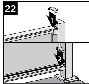
22. Attach corresponding bracket covers over opening in top and bottom rails.
