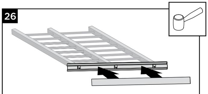
26. Using a mallet, install bottom rail cover onto bottom rail.
