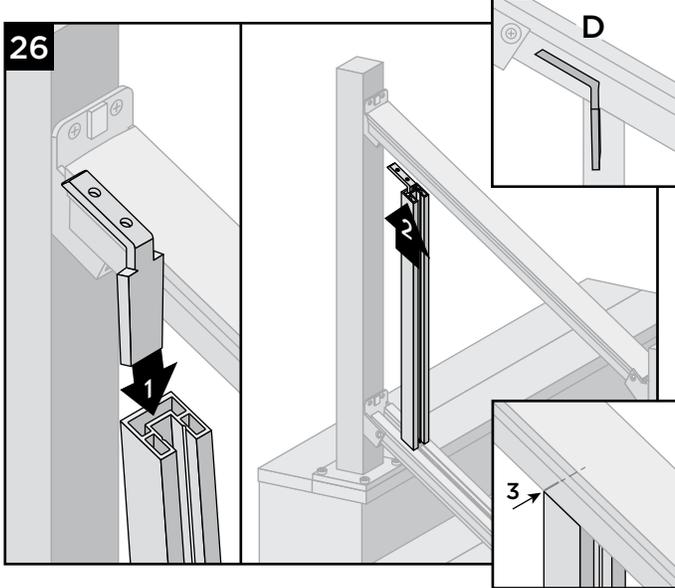
26. Insert L-bracket into vertical and place bracket into channel of top rail. Ensure that vertical is seated fully flush with top rail, bracket is in the channel, and vertical is aligned with mark on rail.
