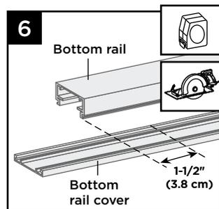
6. Mark and cut bottom rail cover  $1\frac{1}{2}$ " (3.8 cm) shorter than bottom rail.
