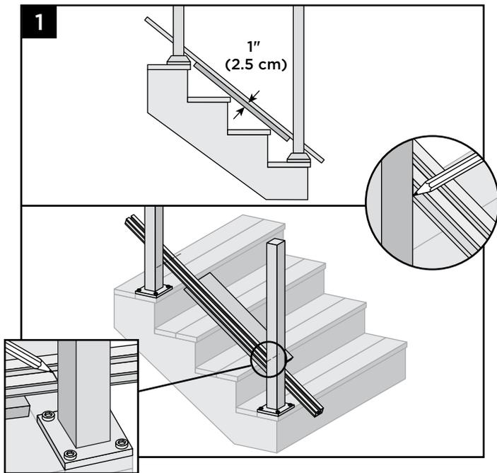
1. Place a 1" deck board along the nose of the stair tread, then lay the bottom stair rail on top of the deck board. Use the lower and upper stair post to determine the length of the bottom stair rail. At **LOWER STAIR POST**, mark on topside of rail and cut PERPENDICULAR to the rail. At **UPPER STAIR POST**, mark on INTERSECTION/SIDE OF RAIL AND CUT RAIL TO THIS ANGLE.
