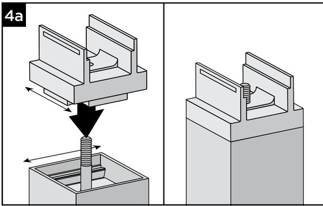
4a. Place the line crossover bracket over the bolt onto the end of the post.
