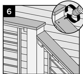
4. Secure boards to top rail using Trex Signature Cocktail Bracket (sold separately). Ensure that there is a bracket at each end of the stair railing section, then space brackets approximately every 24" and attach with 4 screws provided.
