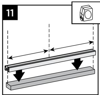
11. Place universal rail (remembering to orient this properly so that when flipped over, the universal rail will accept the glass panel and panel support molding), on the 2 x 4, centered.
