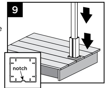
10. Attach bottom guide block using one 10 x 1" self-tapping screw (*provided*) in notch to lock guide block onto post.
