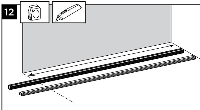
12. Cut both bottom sill gasket and top head gasket to the same length of glass panel.
