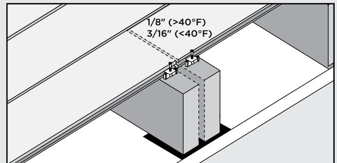
**NOTE:** Optional - Gap joist framing 1/8" - 3/16" to allow for water drainage.
