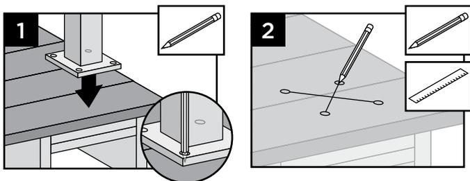
1. Before attaching post to deck, locate placement of post and mark desired bolt locations.
