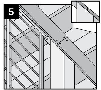
3. Place deck boards over top rails. **DO NOT** use Enhance deck boards for top rail. PLACE DECK BOARD ON TOP RAIL TO CHECK FOR PROPER FIT AND RAIL CLEARANCE AT BRACKET LOCATIONS. DECK BOARD MAY REQUIRE EITHER A NOTCH CUT ON THE UNDERSIDE OR SLIGHT PLANING ON THE UNDERSIDE TO ALLOW DECK BOARD TO CLEAR TOPS OF BRACKETS AND SIT FLUSH ON TOP OF POSTS AND RAILS. Attach boards on each post with Trex-recommended composite screws (quantity of 2 per each post/board end).
