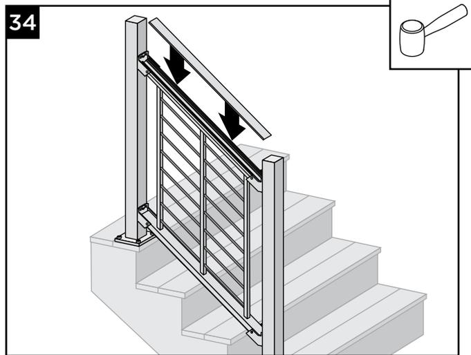
34. Using a mallet, install top rail cover.
