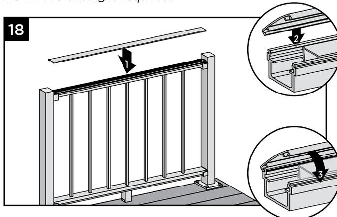
18. Attach "crowned" upper rail cover to upper rail by aligning cover on one side of rail. Then starting from one end of rail, snap cover onto opposing slot working down length of rail. **GENTLE** tapping with a **rubber mallet** may facilitate fastening.
