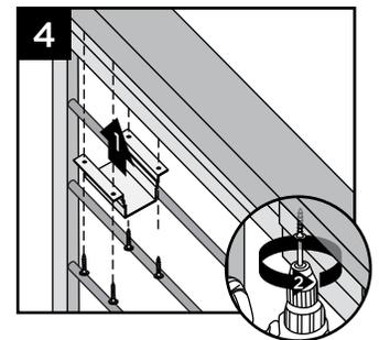
**NOTE: Pre-drilling before attachment is recommended.**
