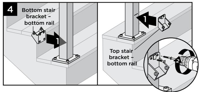
4. Center lower stair bracket on post below the marked line and attach using two #10 x 5/8" self-tapping screws (provided). In some cases it may be difficult to attach the stair bracket on the lower stair post. Recommend using a 90° drill adapter or loosen the post to get access to the lower bracket screw holes.
