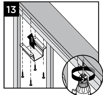
**NOTE: Pre-drilling before attachment is recommended.**
