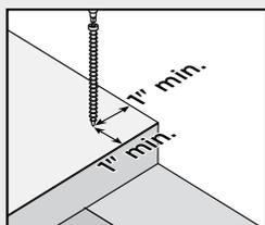
Install fasteners at a 90° angle (perpendicular to the board).
