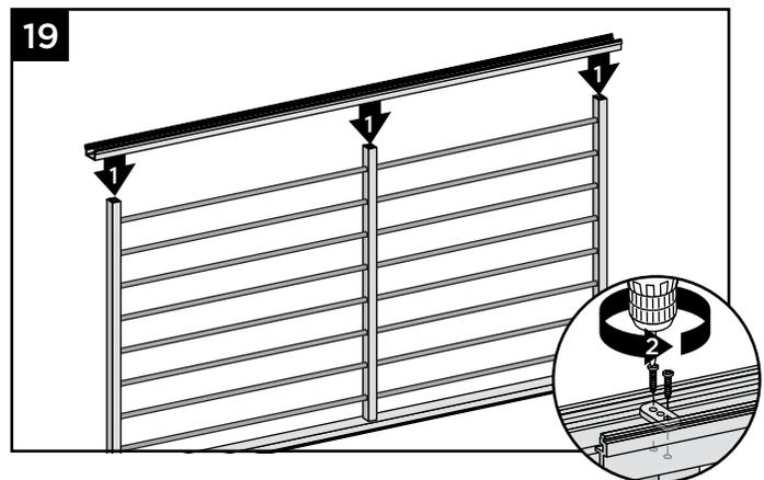
19. Install top rail to all vertical and end supports using HZ spacer and screws provided. HZ spacer should be oriented so the ribbed side of the spacer is not showing.
