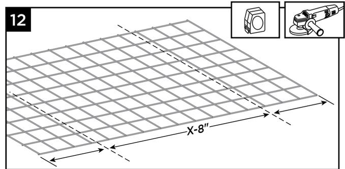
12. Cut mesh panel to this measurement, again cutting equal distances from each side so mesh is centered.
