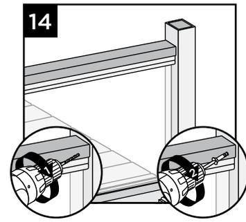
14. Pre-drill a pilot hole and toenail 2-1/2" (64 mm) composite deck screw (*not provided*) at each end of the 2 x 4 into post on back side (side not facing decking).
