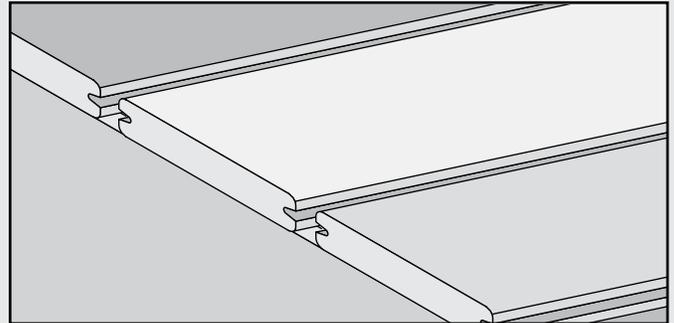
If installing in localities prone to large temperature shifts within a 24-hour period, and installing Trex Universal Hidden Fasteners, pre-drill and toenail a screw (use same screw used in hidden fasteners) at an angle in groove at both ends (at least 1" (25mm) from board end) and center of each board.
