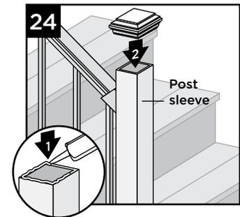
24. Attach post caps to post sleeves using external grade PVC construction adhesive (apply adhesive on the inside self-centering/corner tabs).
