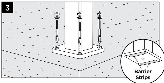
3. Insert the (2) stainless steel barrier strips under the mounting bolt holes. Use appropriate shims if posts are not plumb. Secure post mount with the four expansion anchors, washers and nuts.
