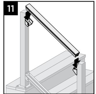
11. Set top stair rail into top stair rail brackets.
