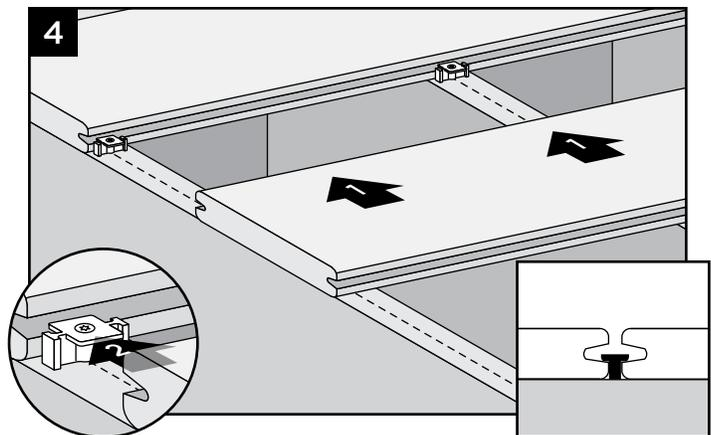
4. Install next board against installed hidden fasteners. Some slight force (using a rubber mallet) to seat next board against fasteners may be required.
