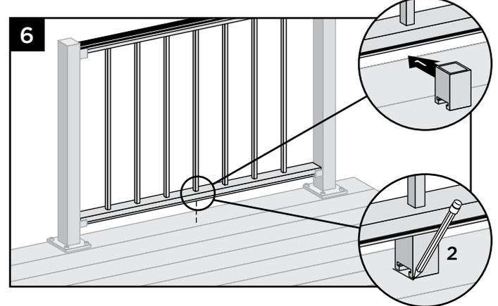
6. Temporarily place panel onto brackets. To ensure correct location, place Foot Block under center of bottom panel rail. Mark to provide placement location of base.
