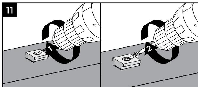
11. Place base (smaller side facing down) on decking surface. Pre-drill using a 3/16" bit. Attach base of Foot Block using one screw at an angle through base and into decking.
