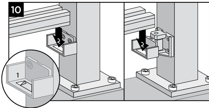
10. Place adhesive strips (provided) into bottom rail brackets, and then place bottom rail into brackets. Using a 3/8" drill bit, drill weep holes through center of bottom rail channel at 4 evenly spanned locations to allow for water drainage.
