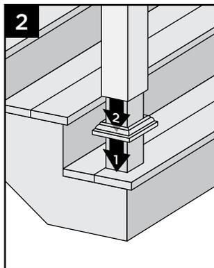
*NOTE: Shims can be used to plumb post sleeves.*
