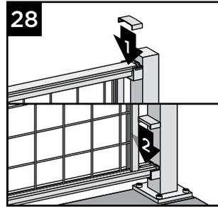
28. Attach corresponding bracket covers over opening in upper and bottom rails.
