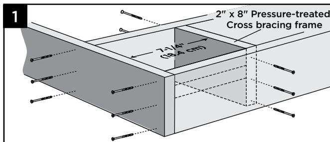
1. Install 2" x 8" (5.1 cm x 20.3 cm) cross bracing frame in between joists at 7-1/4" (18.4 cm). Attach a total of twelve 3" (7.6 cm) pressure-treated compatible screws (not provided).
