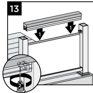
13. Place inverted universal rail with 2 x 4 attached over RSBs and glass panel. Attach universal rail to RSB's with three self-drilling screws provided (use three outer holes; do not use hole in RSB that is closest to post).
