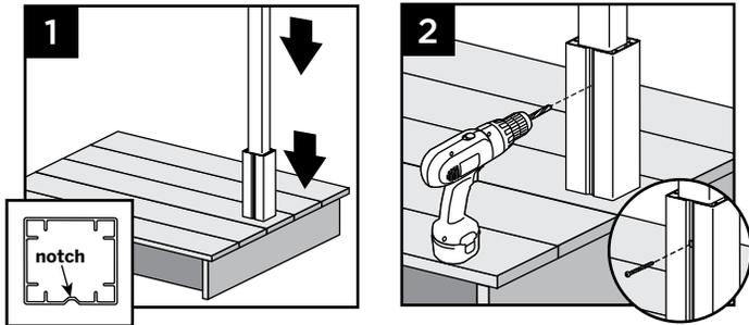
1. Place or rest bottom aluminum guide block on bottom of post. Place guide on post so that notch is on a side that does not require railing to be attached.
