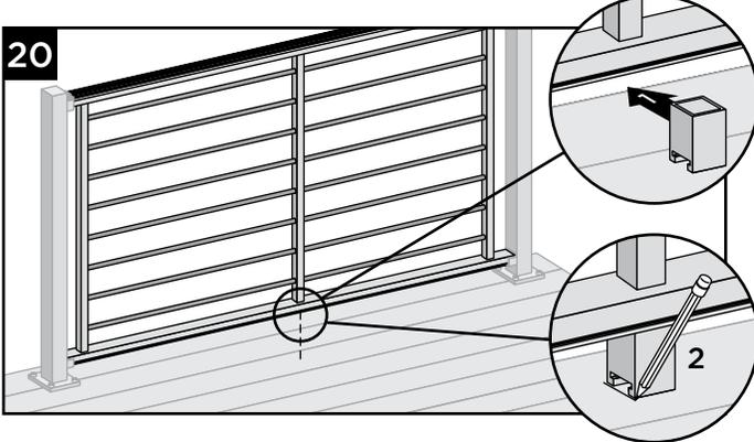
20. Temporarily drop rod rail panel into brackets. To ensure correct location, place Foot Block under center of bottom panel. Mark to provide placement location of base. Once marked remove panel.
