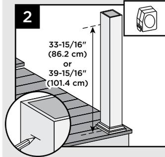
2. Measure up from decking surface 33-15/16" (86.2 cm) for 36" (92 cm) rail height or 39-15/16" (101.4 cm) for 42" (107 cm) rail height. Mark with light line.
