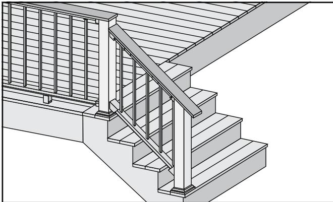
» *THE DECK BOARD USED IN TREX SIGNATURE COCKTAIL RAILING WILL NEED TO TERMINATE AT THE TOP OF THE POST AS SHOWN ABOVE. THE DECK BOARD WILL HAVE TO BE TOENAILED INTO THE SIDE OF THE POST IN THESE AREAS USING 2 APPROPRIATE COMPOSITE DECKING SCREWS - PRE-DRILLING IS RECOMMENDED.*
