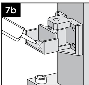
7b. Put a dab of silicone in the basket of the bottom of the bracket to prevent rattle.
