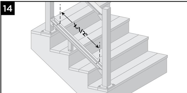
14. Measure distance between marked lines on bottom rail and subtract 1/2" from this measurement.
