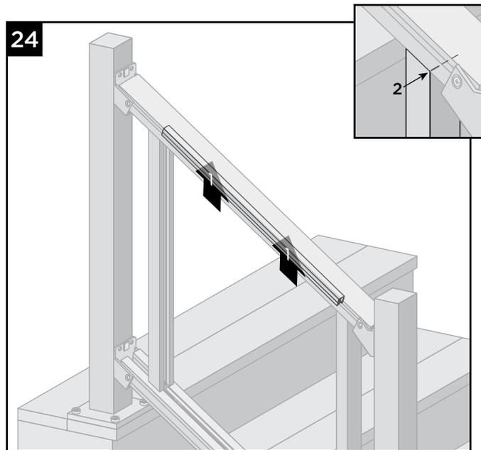
24. Gently tap gasket into channel of top rail. Make sure that vertical is properly aligned with mark on top rail to ensure this is seated in correct location **BEFORE** attaching L-bracket.
