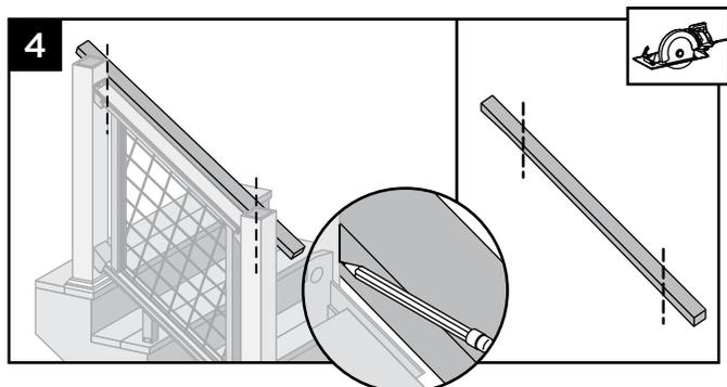
4. Place 2 x 4 beside top rail. Mark and cut (both ends need to be cut on an angle for proper fit).
