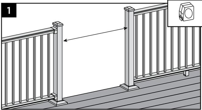
1. Measure opening between posts (gates can be customized to fit nearly any opening up to 48" [1219 mm] wide).
