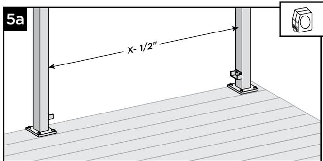
5a. Measure distance between posts (X), and subtract 1/2" for bracket clearance.
