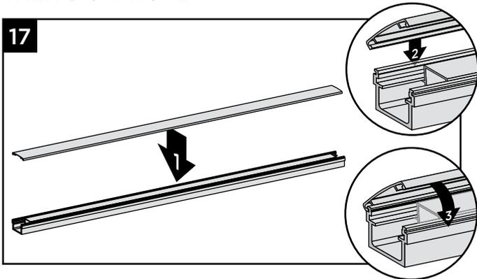
17. Attach “crowned” upper stair rail cover to upper stair rail by aligning cover on one side of rail. Then starting from one end of stair rail, snap cover onto opposing slot working down length of stair rail. **GENTLE** tapping with a **rubber mallet** may facilitate the fastening.
