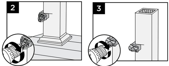
2. Position RSBs with adapter (flat side DOWN) for lower rail, mark and pre-drill screw holes with 1/8" (3 mm) drill bit on post.
