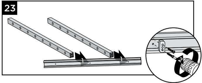
23. Install lowest end vertical and all intermediate verticals to bottom rail using ST Wedge Spacer and screws provided.
