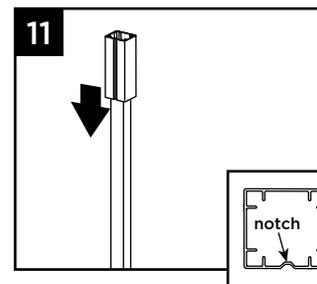
11. Location of top guide block will vary slightly depending on type and height of railing being installed. Determine this measurement and place top guide block in location where top bracket for desired railing would be approximately on center of the top railing bracket location.
