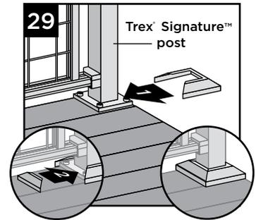
29. Attach provided post skirt to bottom of posts when using Trex Signature posts.
