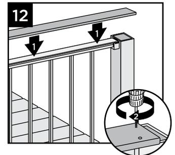
13. Secure boards to top rail using Trex Signature Cocktail Bracket (sold separately). Ensure that there is a bracket at each end of the railing section, then space brackets approximately every 24" and attach with 4 screws provided.
