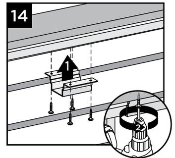
**NOTE:** Pre-drilling before attachment is recommended.
