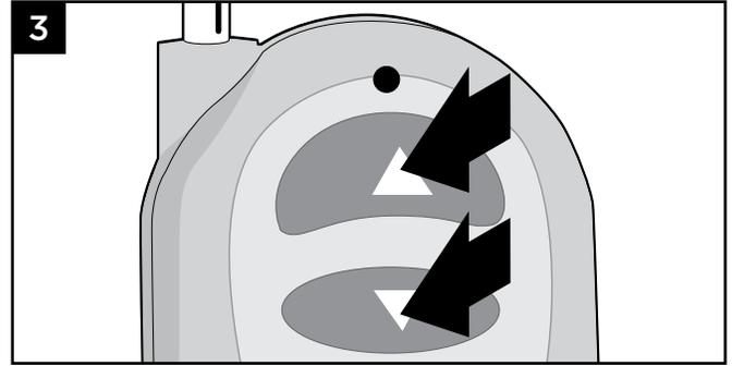
3. Press and hold both the up and down arrow on the dimmer remote simultaneously.
