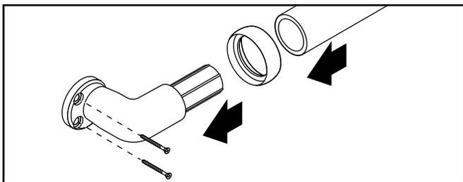
1. If required, cut railing to proper length based on location of wall return(s) or attachment to other components.
