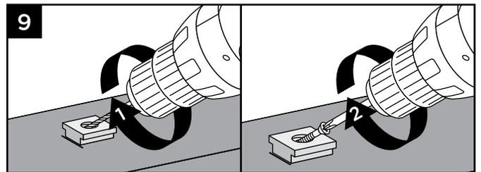
9. Remove bottom rail from lower brackets. Place base (smaller side facing down) on decking surface. Pre-drill using a  $3/16"$  bit. Attach base of Foot Block using one screw at an angle through base and into decking.
