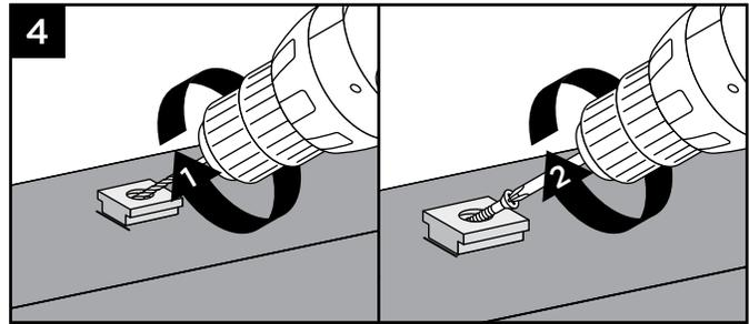
4. Place base (smaller side facing down) on decking surface. Pre-drill using a 3/16" bit. Attach base of Foot Block using one screw at an angle through base and into decking.
