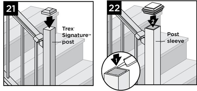
21. Attach post caps to Trex Signature posts (use of **rubber mallet** may be required for secure attachment).
