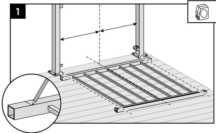
1. Position panel between posts and align with bottom bracket. Align center baluster with middle of span between posts (this will allow for equal spacing between end balusters and each post). Mark bottom and top rail at each end.
