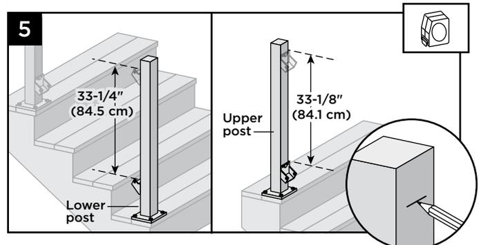
5. On Lower Post: From top of lower bracket, measure up and mark with light line (33-1/4" for 36" rail; 39-1/4" for 42" rail). On Upper Post: From top of lower (upper) bracket, measure up and mark with light line (33-1/8" for 36" rail; 39-1/8" for 42" rail).
