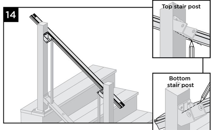
14. On top stair post location, mark **UNDERSIDE** of upper rail. On bottom stair post location mark **TOPSIDE** of upper rail at angled intersection inside the bracket.
