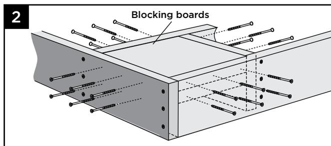
2. Install two 2" x 8" (5.1 cm x 20.3 cm) boards as blocking under post location. Securely attach blocking using a total of twenty-four 3" (7.6 cm) pressure-treated compatible screws (not provided).
