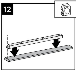
13. Secure deck board to Select top rail with 3/4" screws provided approximately every 16" on center. Screws are to be installed inside of the baluster holes into the decking board.
