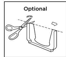
13. Use scarf cut for posts where two deck boards meet.
