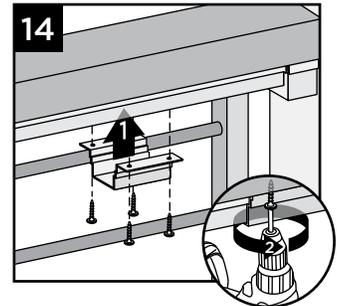
**NOTE:** Pre-drilling before attachment is recommended.
