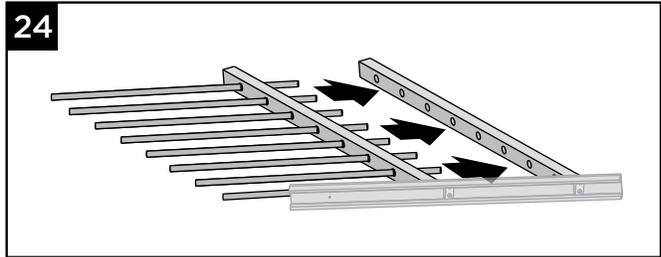
24. Slide rods into lower end and all intermediate verticals.
