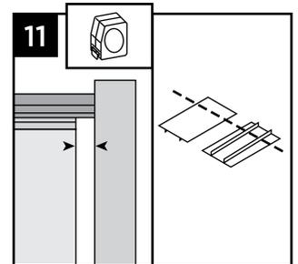
12. Snap spacer into bottom and top rail to hide brackets and create a seamless look.
