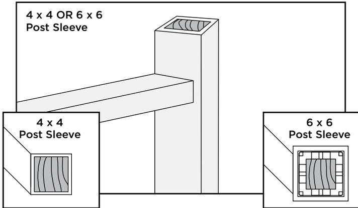
Both 4" x 4" (102 mm x 102 mm) or 6" x 6" (152 mm x 152 mm) post sleeves work well for angles up to 45 degrees. Bottom rail brackets may need to be slightly offset to one side in order to fit properly to hold rail in place. Before attaching bracket to rail, measure and mark to ensure bottom rail remains parallel to upper rail.
