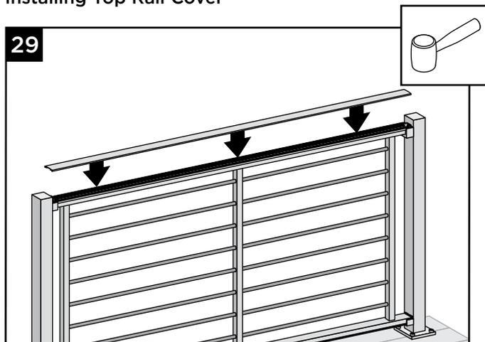
29. Using a mallet, install top rail cover.
