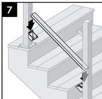
10. Set top stair rail into top stair rail brackets.
