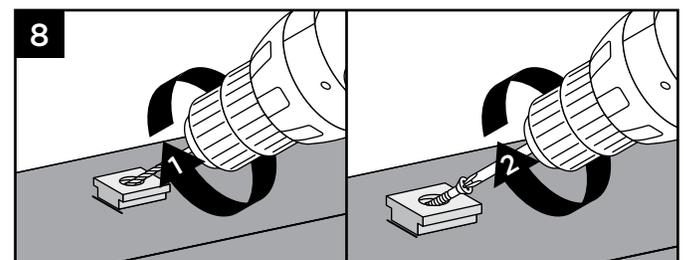
8. Remove bottom rail from lower brackets. Place base (smaller side facing down) on decking surface. Pre-drill using a 3/16" bit. Attach base of Foot Block using one screw at an angle through base and into decking.
