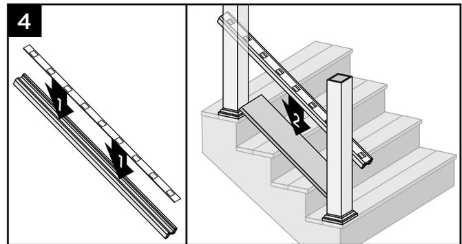
4. Snap baluster spacer into bottom stair rail and lay bottom stair rail on top of the deck board.
