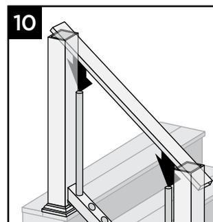
9. Place two balusters into lower stair rail at each end closest to the post.
