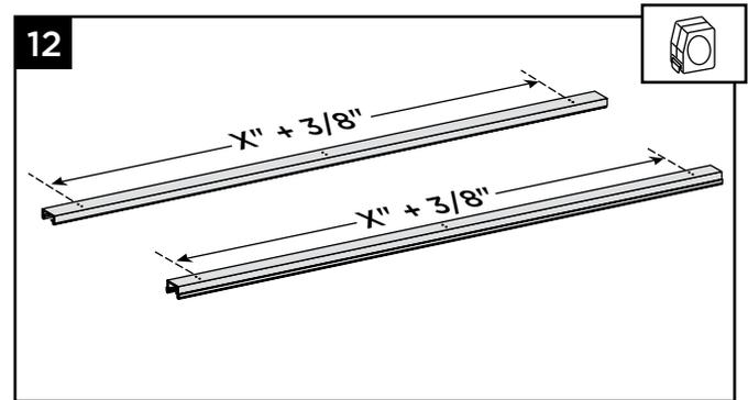
12. Measure the distance between the end (outer) holes (X") on top or bottom rail and add 3/8" to this measurement.
