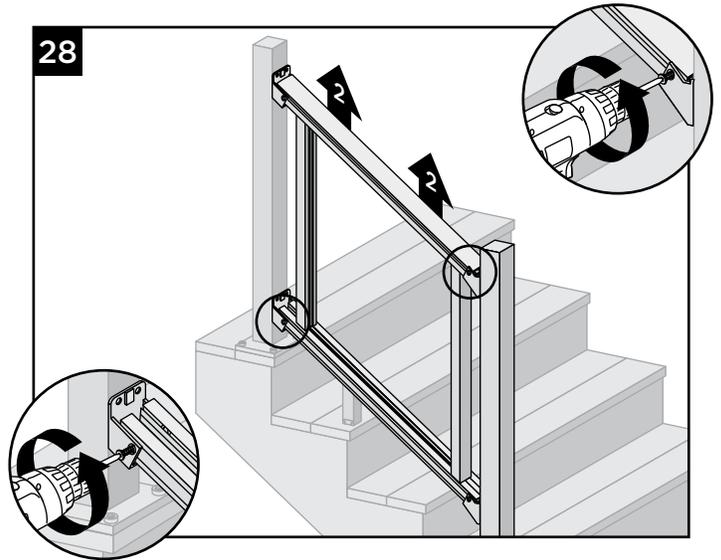
28. Remove the two screws from the brackets that were previously installed in step 9. Remove the railing assembly from the post brackets.
