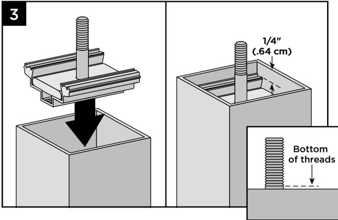
3. Insert assembly (from step 2) into the top of post. Stop when top of v-wedge is about 1/4" into top of post.
