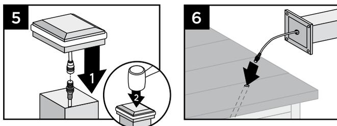
5. Connect the female connector on the post cap light to this wire and, using a rubber mallet, gently tap the cap onto top of post until it is secure.
