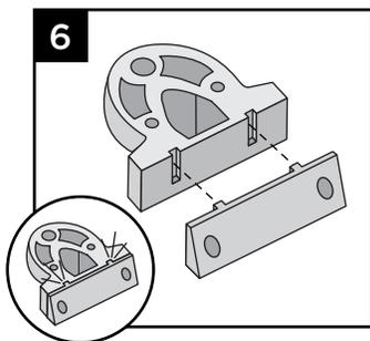
**TIP:** Use a dab of super glue when snapping bracket together. This will help stabilize bracket when installing.
