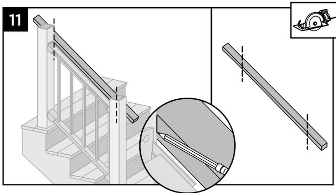
11. Place 2 x 4 beside top rail. Mark and cut (both ends need to be cut on an angle for proper fit).
