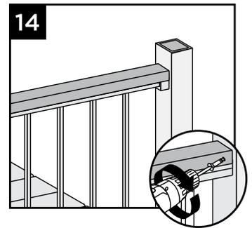
13. Secure 2x4 (to top rail using Trex Signature Cocktail Bracket (sold separately). Ensure that there is a bracket at each end of the railing section, then space brackets approximately every 24" and attach with 4 screws provided.
