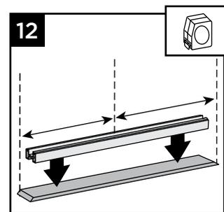
12. Place universal rail on the deck board. Orient this properly so when flipped over, the universal rail will accept the glass panel and panel support molding. Center in both directions to allow final attachment to post.
