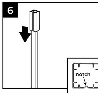
6. Location of top guide block will vary slightly depending on type and height of railing being installed. Determine this measurement and place top guide block in location where top bracket for desired railing would be approximately on center of the top railing bracket location.
