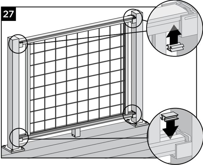
27. Cut snap-in channel filler to correct length at each location and install into channels of bottom and top rails. Use of a rubber mallet may assist with this step. **DO NOT** attempt to cut short snap in pieces with a miter saw. Use an angle grinder or hack saw only.
