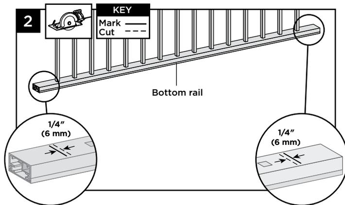
2. Using a saw equipped with a non-ferrous metal blade, cut each end of bottom rail and bottom rail insert  $1/4''$  (6 mm) shorter than mark on each end to allow for fit into bottom rail brackets.
