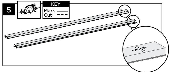
5. Cut both bottom and top rail to length as determined in previous step.
