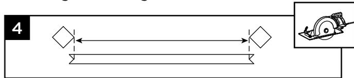
4. Measure from corner-to-corner between posts. Mark 45° cuts on rails with template on assembly tool. Center of “V”'s is the distance from corner-to-corner for posts.
