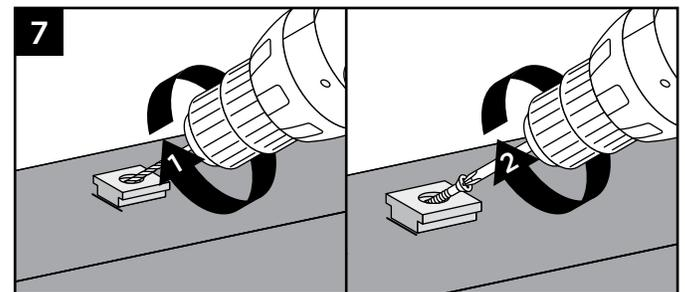
7. Remove railing panel and place base (smaller side facing down) on decking surface. Pre-drill using a 3/16" bit. Attach base of Foot Block using one screw at an angle through base and into decking.
