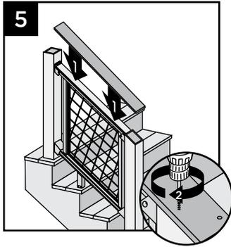
6. Secure boards to top rail using Trex Signature Cocktail Bracket (sold separately). Ensure that there is a bracket at each end of the stair railing section, then space brackets approximately every 24" and attach with 4 screws provided.
