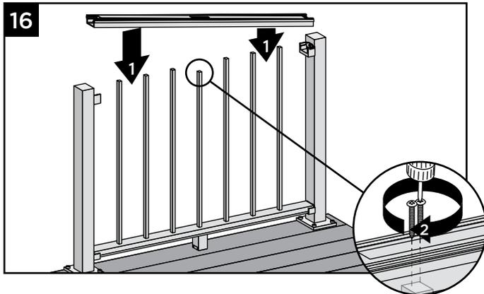
16. Working from one end of upper rail, snap balusters into upper rail working down length of rail. Fasten center baluster into center slot using two #8 x 1-1/4" (3.2 cm) screws (provided).
