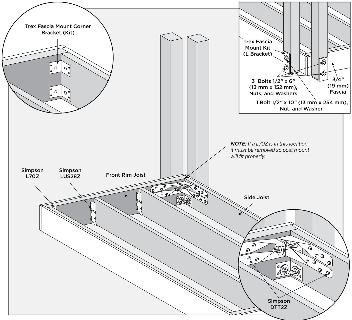
**NOTE:** If a L70Z is in this location, it must be removed so post mount will fit properly.
