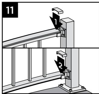
13. Attach post caps to Signature posts. (A **rubber mallet** may be required for secure attachment.)
