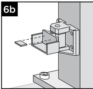
6b. Break or cut the bottom tab off the bottom brackets.
