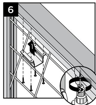
6. Secure 2 x 4 to top rail using Trex Signature Cocktail Bracket (sold separately). Ensure that there is a bracket at each end of the railing section, then space brackets approximately every 24" and attach with 4 screws provided.
