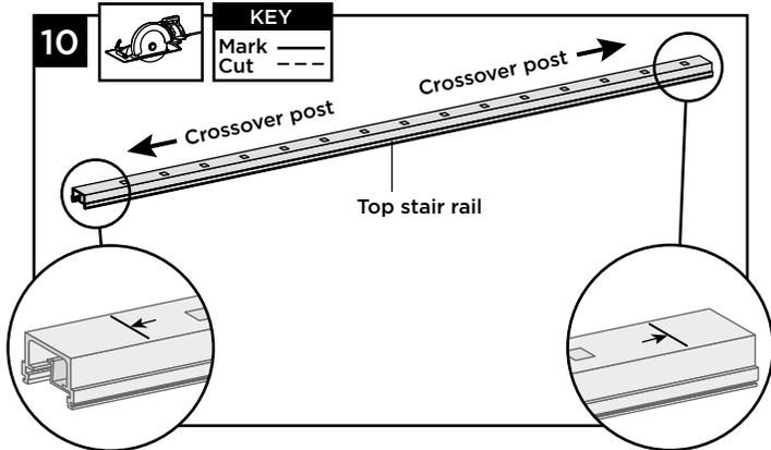
10. Cut each end of the top stair rail along with rail insert on the mark line to allow for fit into the crossover post bracket on each side.
