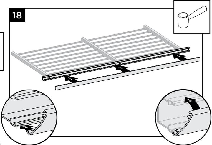
18. Align cover on one side of bottom rail in slot on side of rail. If using tabbed brackets, the bottom rail cover will also have to be centered on bottom rail to allow for fit into tabbed bracket. Then starting from one end of rail snap cover onto opposing slot working down the length of rail. In some cases, GENTLE tapping with a rubber mallet may facilitate fastening.
