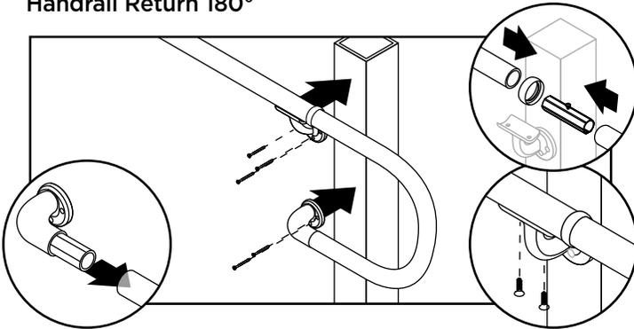
**NOTE:** Ramp application shown here. (Appropriate angle elbow also required for stair applications.)
