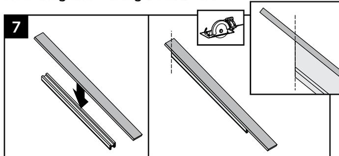
7. Using the cut top rail as template, cut deck board at upper post location at same angle as the top rail. Leave a generous amount of deck board material at lower post location as this will allow for overhang and can be cut later.
