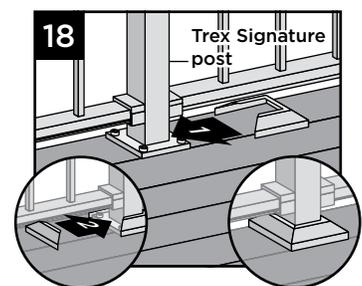
18. Attach provided post skirt to bottom of posts when using Trex Signature posts.
