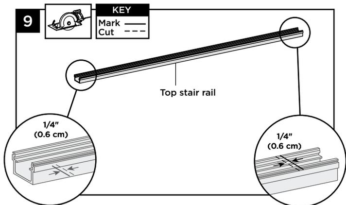
9. Cut each end of top stair rail and top rail cover  $\frac{1}{4}$ " (0.6 cm) shorter than mark to allow for fit into top stair rail bracket.
