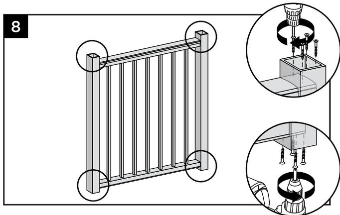
8. Secure posts to panel with four #8-18 short self-tapping screws (*provided*) in each location.
