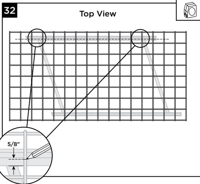
32. At inside of top rail measure **UP** 5/8" and mark mesh at this location. Do this at opposite end of mesh panel/top rail. Using straight edge, mark **MESH ONLY** at all intersection points.
