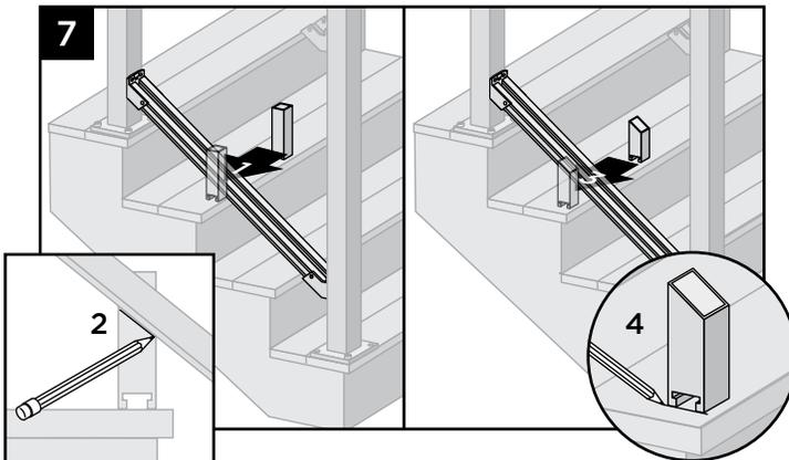
7. Temporarily set bottom stair rail into brackets. To ensure proper location place Foot Block towards the nose of the stair tread along the side of the bottom rail. Mark location of angle on Foot Block and cut on mark. Then place Foot Block under the center of the bottom rail. Mark placement location
