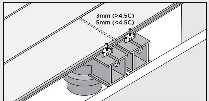
**NOTE:** Hidden Fasteners MUST be used at every joist.
