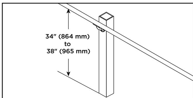
2. The handrail system top rail should be 34" (864 mm) to 38" (965 mm) above the surface. However, verifying height requirements with local building code officials before installing is important as codes vary in different areas.\*
