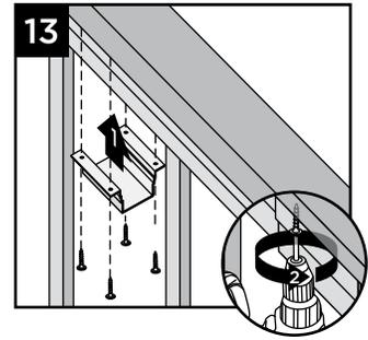
**NOTE:** Pre-drilling before attachment is recommended.
