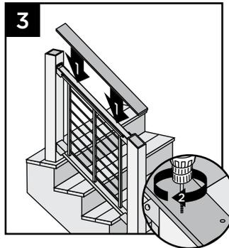
6. Where deck board terminates at upper post, PREDRILL and toenail two approved composite deck screws as shown into post, being careful to avoid hitting stair bracket.
