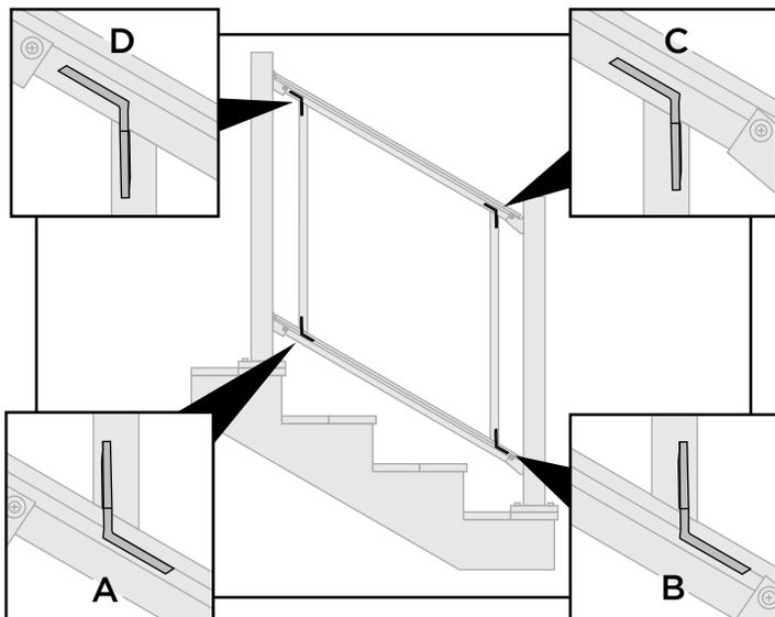
Above is an overall image showing bracket orientation. The next steps will show in detail how to attach them. Refer to corresponding letters in the following steps.
