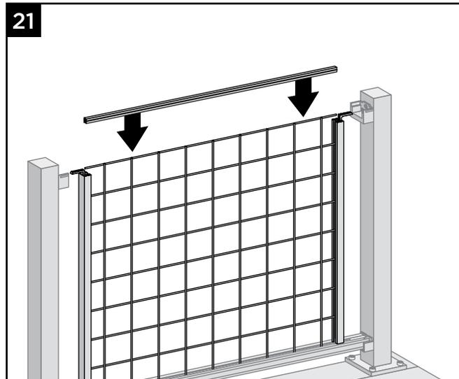
21. Install cut gasket onto top of mesh panel. Make sure gasket is fully seated onto mesh.
