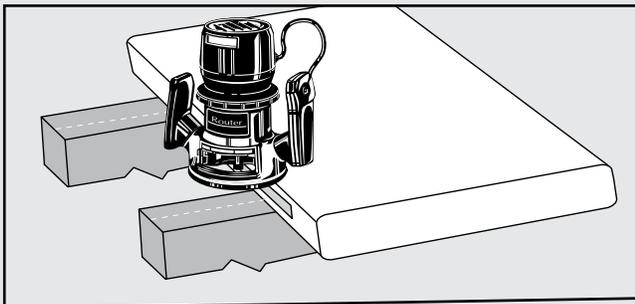
Using a Trex routerbit with standard router:
