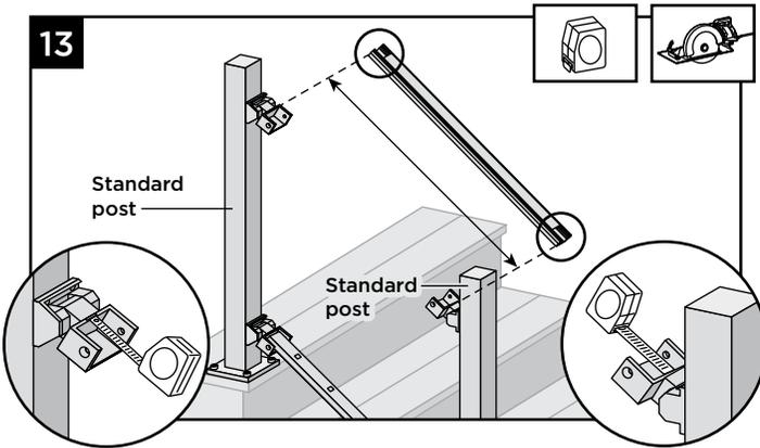
13. Cut top rail along with rail insert to the measurement between the top stair swivel brackets. For standard post to standard post configurations this would be same dimensions as that of the bottom stair rail.
