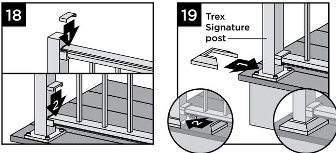
18. Attach corresponding bracket covers over opening in upper and bottom rails.
