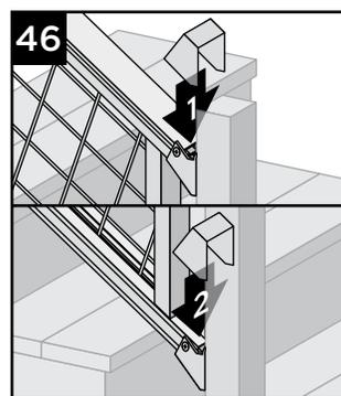
46. Attach corresponding bracket covers over opening in upper and bottom rails.
