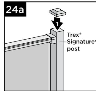
24a. Attach post caps to Trex Signature posts. (Use of **rubber mallet** may be required for secure attachment.)
