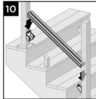
10. Set bottom stair rail into bottom stair rail brackets.
