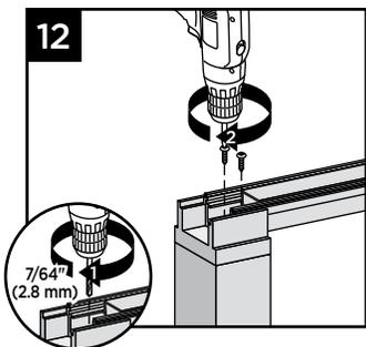
**NOTE:** Pre-drilling is recommended (7/64" [2.8 mm] drill bit) for attachment of railing to bracket.
