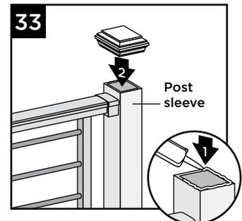
33. Attach post caps to post sleeves using external grade PVC construction adhesive (apply adhesive on the inside self-centering/corner tabs).
