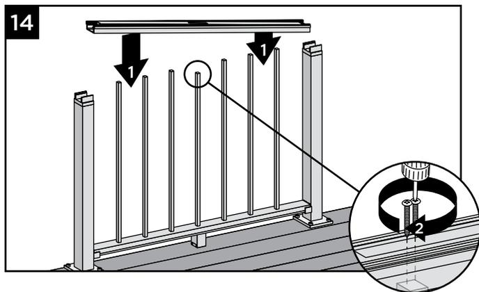
14. Working from one end of upper rail, snap balusters into upper rail working down length of rail. Fasten center baluster into center slot using two #8 x 1-1/4" (3.2 cm) screws (*provided*).
