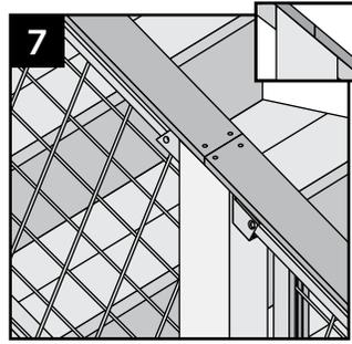
7. Use scarf cut for posts where two deck boards meet.
