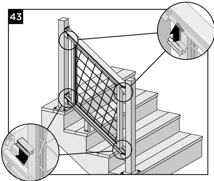
43. Cut snap-in channel filler to correct length and install into channels of bottom and top stair rails. Use of a rubber mallet may assist with this step. **DO NOT** attempt to cut short snap-in pieces with a miter saw. Use an angle grinder or hack saw only.
