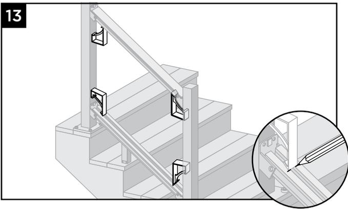
13. Using the long edge of the stair template, mark the location of the end verticals on the upper and lower rails.
