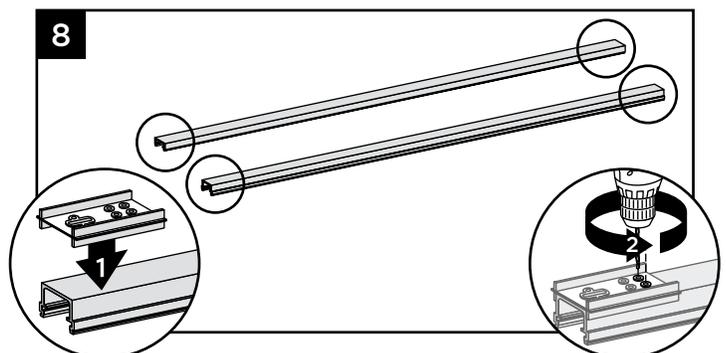
8. Place HZ template at end of top and bottom rails. Pre-drill pilot holes (using a  $\frac{7}{64}$ " bit or small punch) at locations.
