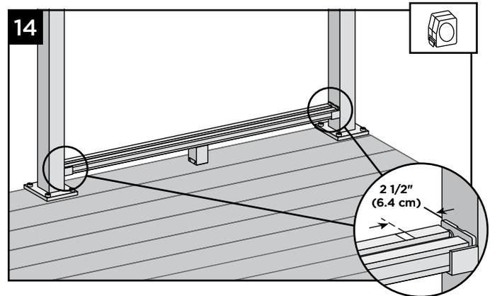
14. For full span installation, make a temporary mark on the bottom rail (example: use removable tape) 2-1/2" from each post. This will allow for glass to be centered between posts on bottom rail.
