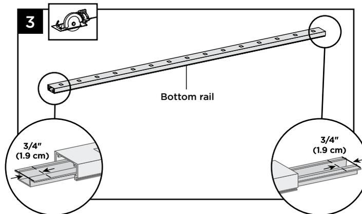
3. Slide rail insert out and cut 3/4" (19 mm) FROM EACH SIDE of insert, then slide back inside rail and center.
