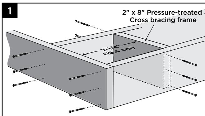
1. Install 2" x 8" (51 mm x 203 mm) cross bracing frame in between joists at 7-1/4" (184 mm). Attach a total of twelve 3" (76 mm) pressure-treated compatible screws (not provided).
