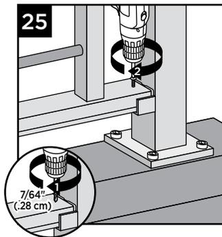
25. If using tabbed lower brackets, using a 7/64" (0.28 cm) drill bit, pre-drill at marked location for attachment of railing to bracket. Attach bottom rail to bottom brackets by using one self-tapping screw (provided) for each bracket. No screws are required if using the tabless lower bracket.
