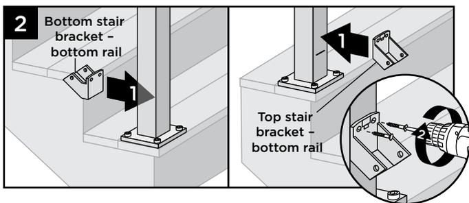
2. Center lower stair bracket on post above the marked line and attach using two self-tapping screws (provided). In some cases it may be difficult to attach the stair bracket on the lower stair post. **A 90° cordless drill is recommended to attach screws in this area.**
