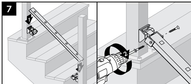
7. Set bottom stair rail into bottom stair rail brackets. Attach bottom stair rail to bottom stair bracket using two self-tapping screws (*provided*) on each side of bracket.
