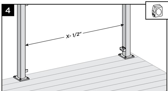
4. Measure distance between posts (X), and subtract  $\frac{1}{2}$ " for bracket clearance.
