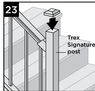
23. Attach post caps to Trex Signature posts (use of **rubber mallet** may be required for secure attachment).
