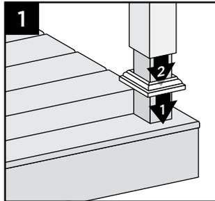
**NOTE:** Shims can be used to plumb post sleeves.
