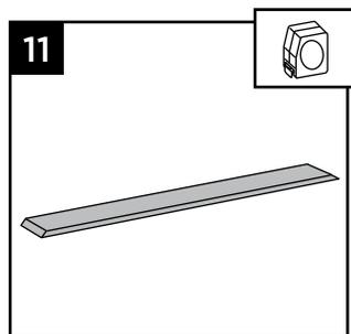
11. Place inverted deck board (place top side of deck board down) on clean, flat surface.
