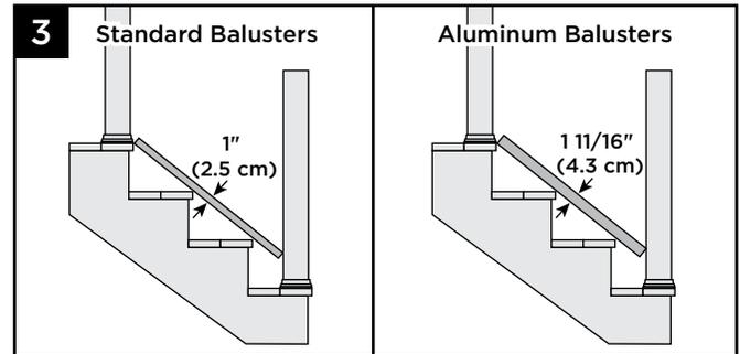
3. If using standard balusters, place a 1" (254 mm) deck board on the nose of the stair tread. If using aluminum balusters, use a scrap piece of wood measuring at least 1-11/16" thick, and place on the nose of the stair tread.
