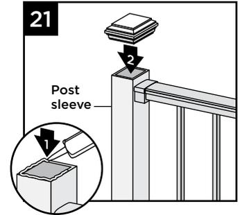
21. Attach post caps to post sleeves using external grade PVC construction adhesive (apply adhesive on the inside self-centering/corner tabs).
