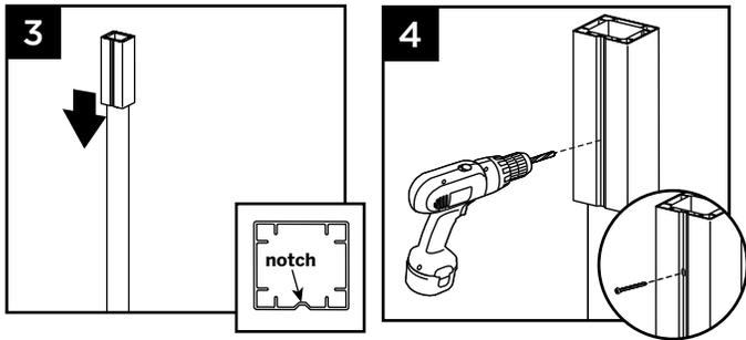
3. Location of top guide block will vary slightly based on type and height of railing being installed. Determine this measurement and place top guide block in location where top bracket for desired railing would be approximately on center of the top railing bracket location.
