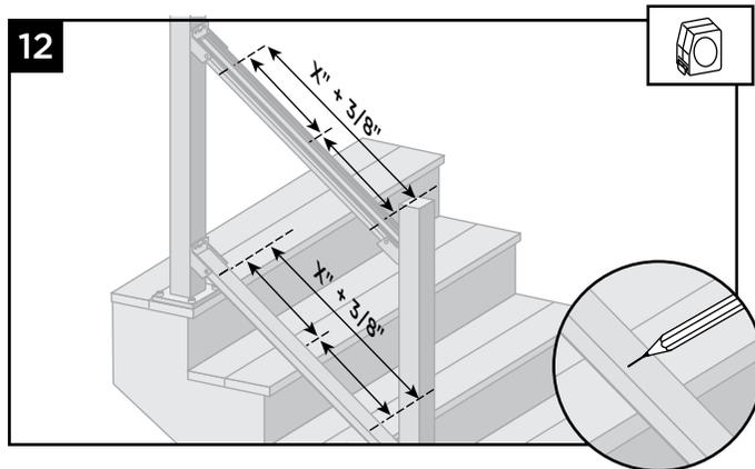
12. Measure and mark the mid-line (6' sections) of the two end marks of the top and bottom rail. Take that measurement and add  $\frac{3}{8}$ " for rod length in next step.
