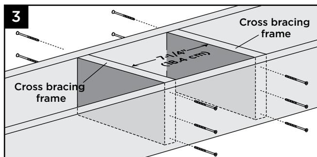
3. Install two 2" x 8" (51 mm x 203 mm) cross bracing frames in between joists at 7-1/4" (184 mm). Attach a total of twelve 3" (76 mm) pressure-treated compatible screws (not provided).
