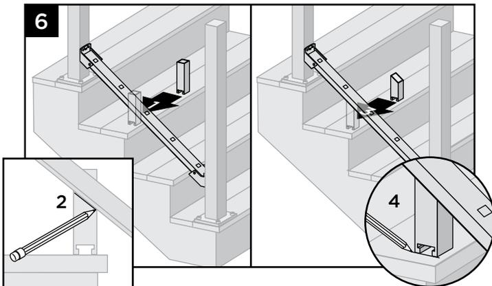
6. Temporarily set bottom rail in bottom brackets, and place Foot Block towards the nose of the stair tread along the side of the bottom rail. Mark location of angle on Foot Block and cut on mark. Then place Foot Block under the center of the bottom rail. Mark placement location of the base. Remove lower rail.
