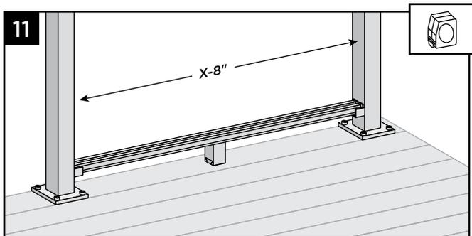
11. If not installing full span, mesh will require cutting from equal distance on each side. Measure distance between posts and subtract 8".
