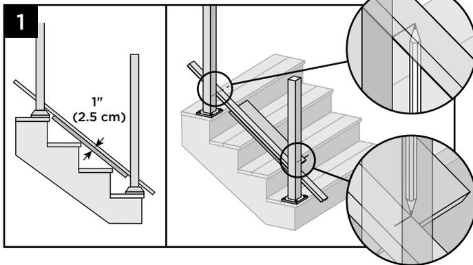
1. Place a 1" deck board on the nose of the stair tread, then lay the bottom stair rail on top of the deck board. Use the lower and upper stair post to set the size of the lower stair rail. On **UPPER STAIR POST**, mark from underside of bottom rail. On **LOWER STAIR POST**, mark from top side of bottom rail.
