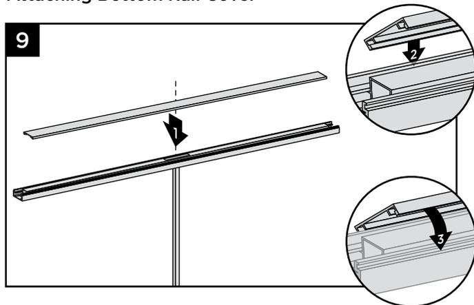
9. Align cover on one side of bottom rail in slot on side of rail. If using tabbed brackets, the bottom rail cover will also have to be centered on bottom rail to allow for fit into tabbed bracket. Then starting from one end of rail snap cover onto opposing slot working down the length of rail. In some cases, **GENTLE** tapping with a **rubber mallet** may facilitate fastening.
