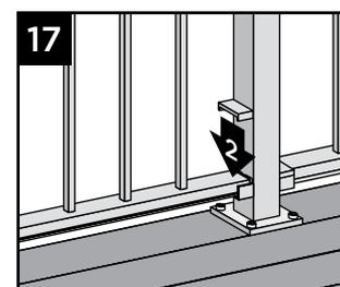
17. Attach corresponding bracket covers over opening in bottom rails.
