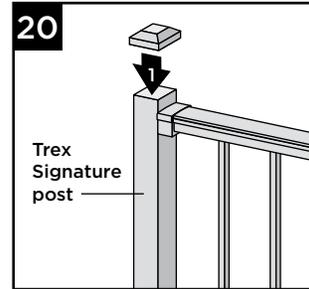
20. Attach post caps to Trex Signature posts. (Use of **rubber mallet** may be required for secure attachment.)
