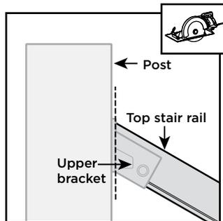
1. Follow all Rod Rail Stair instructions for the assembly of the rod rail stair panel
