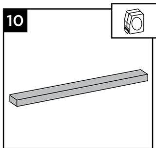
10. Place inverted 2 x 4 on clean, flat surface (place top side down).
