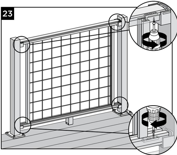
**Attaching L-Brackets to Top and Bottom Rails**
