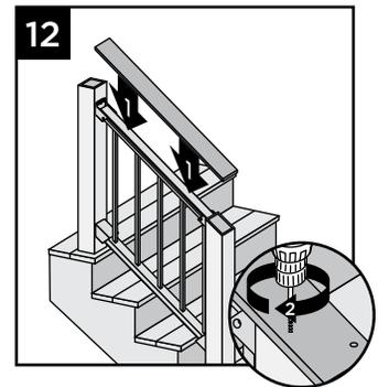
13. Secure boards to top rail using Trex Signature Cocktail Bracket (sold separately). Ensure that there is a bracket at each end of the stair railing section, then space brackets approximately every 24" and attach with 4 screws provided.
