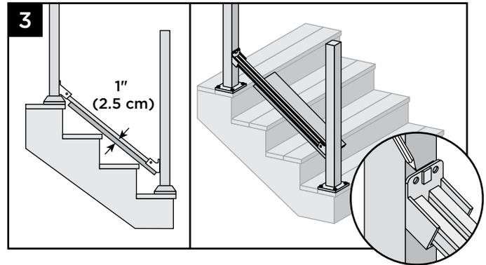
3. With deck board still on nose of stair tread, place brackets on ends of bottom stair rail (but do not attach) and mark posts for bracket locations.
