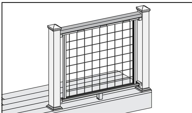
**Important:** Only use with Pressure-treated post, Trex Post Mounts or Trex Joist Mount Post WITH Trex post sleeves. Trex Signature Posts and Joist Mount Posts cannot be used with Mesh Traditional.
