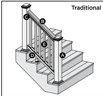
Cutting post sleeves is **NOT** required. Ensure both top and bottom post/post sleeves are tall enough to accommodate top rail and 2 x 4.
