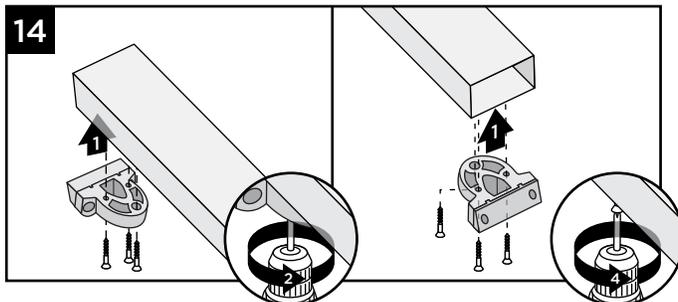
14. On the TOP RAIL, attach the assembled stair brackets to the side WITH the baluster holes. Attach both brackets using three #8-18x1" self-drilling screws (provided).
