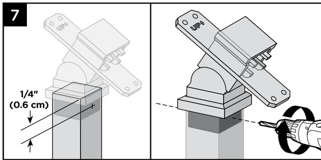
7. Once location/height is determined, center and pre-drill two holes (using a drill bit slightly smaller than that of self-tapping screw diameter) on opposite sides of post, approx. 1/4" (0.6 cm) from top of post. Drill through the post and into the stair crossover swivel bracket on each side.
