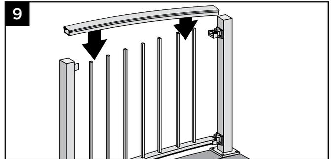
9. Working from one end of upper rail, snap balusters into upper rail, working down length of curved rail.
