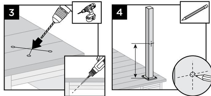
3. Using a 9/16" (14 mm) x 6" (152 mm [or longer]) drill bit, drill a diagonal hole through the decking and blocking. Ensure that the angle will allow wire to not be pinched by support plate under blocking (if using Trex ALPOSTHWDECK mounting kit).
