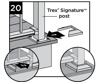
20. Attach provided post skirt to bottom of posts when using Trex Signature posts.
