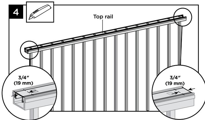
4. Using razor knife or other cutting tool, cut rail insert 3/4" (19 mm) **FROM EACH SIDE**.
