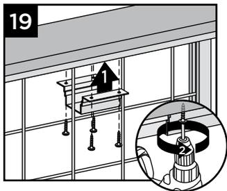
**NOTE:** Pre-drilling before attachment is recommended.
