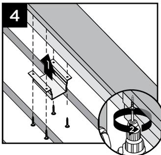
**NOTE:** Pre-drilling before attachment is recommended.
