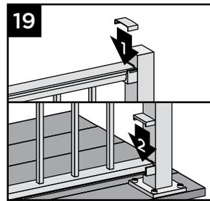
19. Attach corresponding bracket covers over opening in upper and bottom rails.
