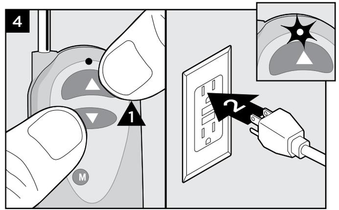
4. With the dimmer arrow buttons held down, plug the transformer back in. The lights should blink once to confirm programming.
