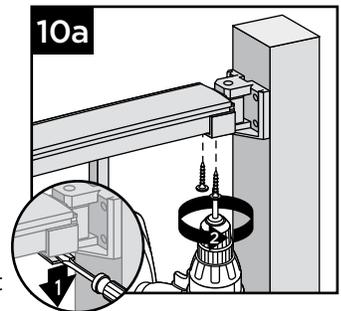
Attach top rail to bracket using two self-tapping screws each side (provided). Screw from the bottom up into the top rail.
