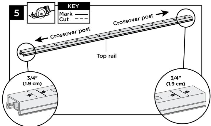
5. Cut each end of top rail 3/4" (1.9 cm) **LONGER** than the mark to allow for fit into the crossover post bracket on each side.
