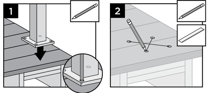
1. Before attaching post to deck, locate placement of post and mark desired bolt locations.
