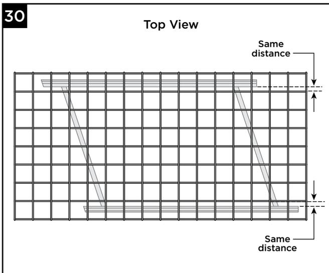
30. Lay mesh panel on top of stair rail assembly and measure so there is equal spacing between mesh panels at both top and bottom rails. Use clamp to hold mesh in place securely once dimensions are set.
