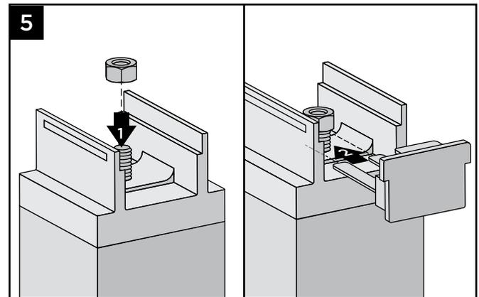
5. Thread the nut onto the bolt. When attaching crossover end cap, slide u-channel on end cap under the nut until cap is flush with the end of the bracket. End cap is for use with the line crossover bracket only (when terminating a rail at a line crossover post).
