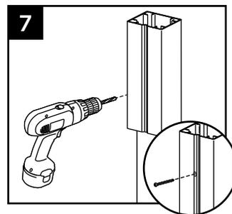
7. Attach top guide block using one 10 x 1" (25 mm) self-tapping screw (provided) in notch to lock guide block onto post.
