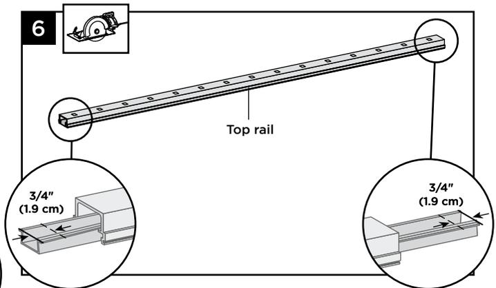
6. Slide rail insert out and cut 3/4" (1.9 cm) **FROM EACH SIDE** of insert, then slide back inside rail and
