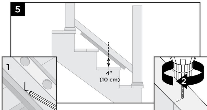
5. Mark approximate location for Foot Block, allowing a measurement of 4" maximum. Invert the bottom rail, and at marked location drill a hole using a 3/16" drill bit in the center of the channel. Foot Block is to be installed at last step.
