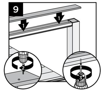
8. Place inverted universal rail onto RSBs. Attach universal rail to RSBs with three self-drilling screws provided (use three outer holes; do not use hole in RSB that is closest to post).
