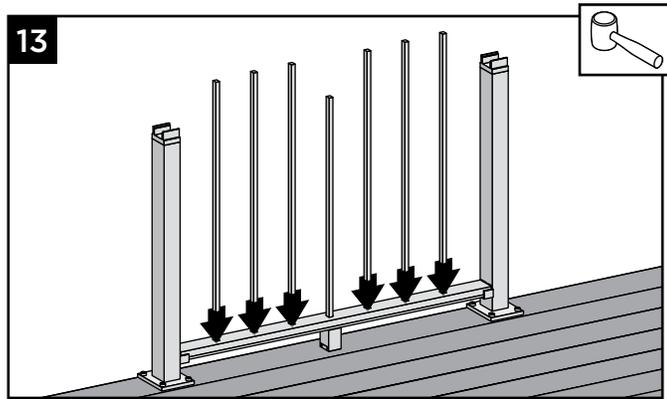
13. Place remaining balusters into holes in lower rail by snapping fully into place. In some cases, **GENTLE** tapping with a **rubber mallet** may facilitate fastening.
