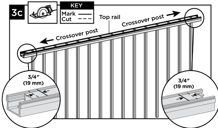
3c. Cut each end of top rail 3/4" (19 mm) **LONGER** than the mark to allow for fit into the crossover post bracket on each side.
