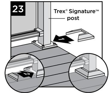
23. Attach provided post skirt to bottom of posts when using Trex Signature posts.
