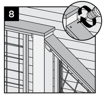
8. Where deck board terminates at upper post, PREDRILL and toenail two approved composite deck screws as shown into post, being careful to avoid hitting stair bracket.
