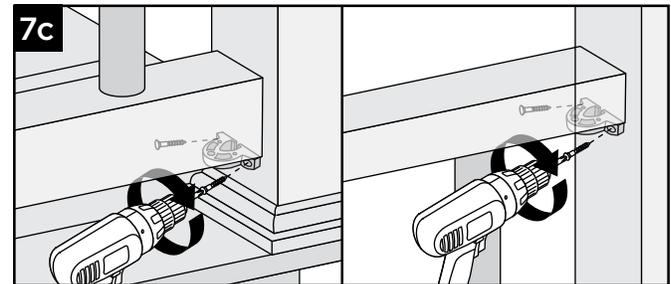
7c. Install both bottom and top brackets on each side to post using two #8-10 x 2" wood screws (provided).
