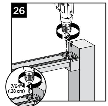
26. Using a 7/64" (0.28 cm) drill bit, pre-drill at marked location for attachment of railing to bracket. Attach top rail to top brackets by using two self-tapping screws (provided) for each bracket.
