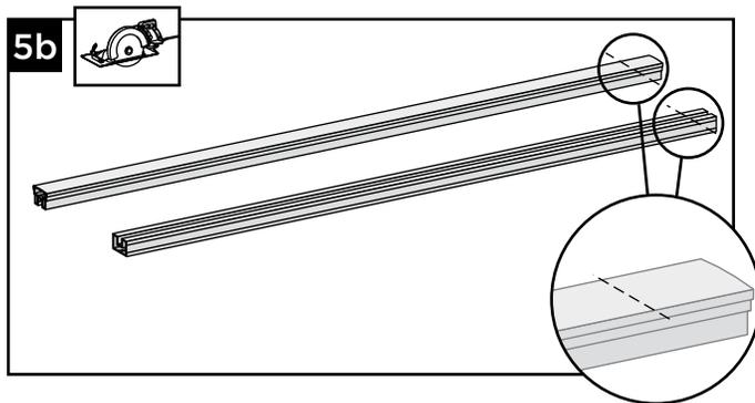
5b. Cut both bottom and top rail to length as determined above.
