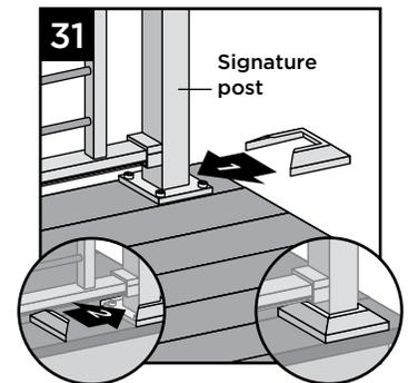
31. Attach provided post skirt to bottom of posts when using Trex Signature posts.
