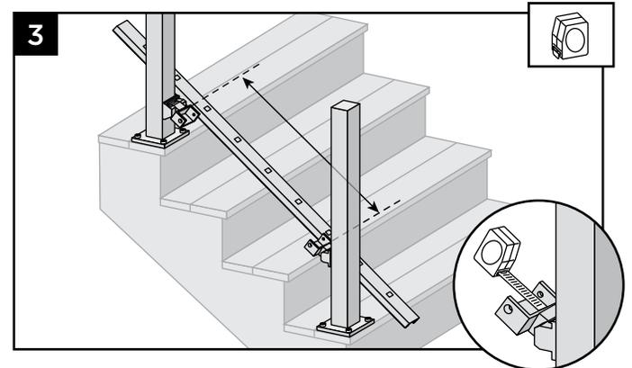
3. With brackets in correct swivel locations, measure distance from inside of swivel bracket to inside of swivel bracket. Ensure that before cutting, balusters holes are parallel and centered in between the posts and also allow for clearance for attachment to brackets. Mark bottom stair rail at each intersection.
