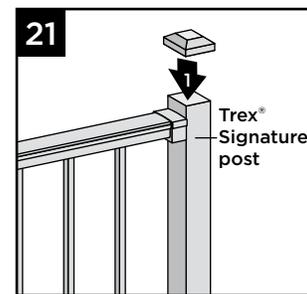
21. Attach post caps to Trex Signature posts. (Use of **rubber mallet** may be required for secure attachment.)
