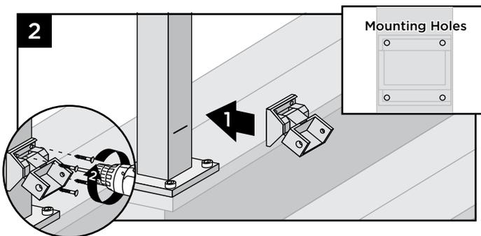
2. Center lower stair swivel bracket on post above the marked line and attach using four self-tapping screws (provided). In some cases it may be difficult to attach the stair bracket on the lower stair post. A 90° cordless drill is recommended to attach screws in this area.
