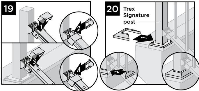
19. Attach corresponding bracket covers over opening in upper and bottom rails.
