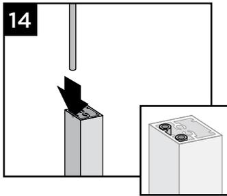
14. Insert anti-rattle strips into the vertical supports.
