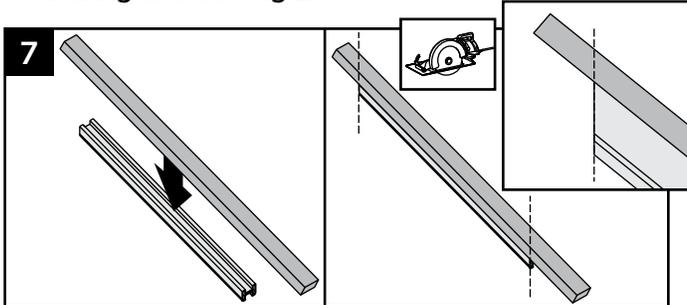
7. Using the cut top rail as template, cut 2x4 at same angle and length of the top rail.
