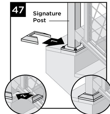
47. Attach provided post skirt to bottom of posts when using Trex Signature posts
