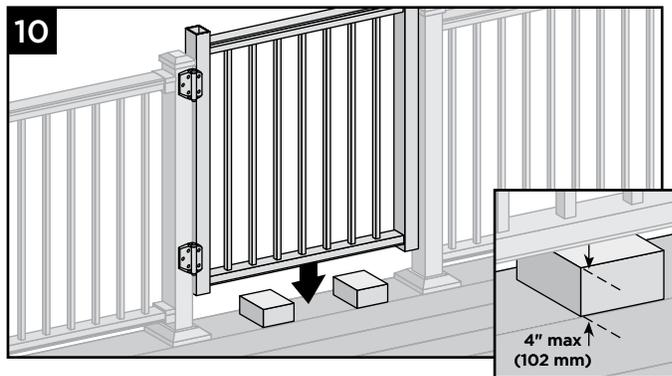
10. Place gate in opening on blocks. Sweep between bottom of gate and top of deck cannot exceed 4" (102 mm) per IRC/IBC code regulations. Ensure bottom gate posts will be high enough to clear skirts on bottom of deck posts.
