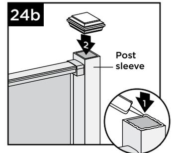
24b. Attach post caps to post sleeves using external grade PVC construction adhesive (apply adhesive on the inside self-centering/corner tabs).
