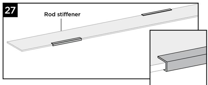
27. Attach tape (qty 6 provided) to alternating sides of the rod stiffener as shown.
