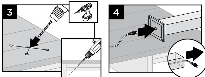
3. Using a 9/16" (14 mm) x 6" (152 mm [or longer]) drill bit, drill a diagonal hole through the decking and blocking. Ensure that the angle will allow wire to not be pinched by support plate under blocking (if using Trex ALPOSTHWDECK mounting kit). (See *Making Connections* section for details.)
