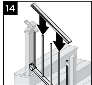
15a. For stair post-to-post configuration, attach top stair rail to top stair bracket (all types) using two self-tapping screws (*provided*) on each side of stair bracket.
