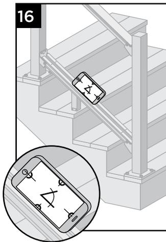
16. Determine the angle of the railing (angle should be between 32-37 degrees).
