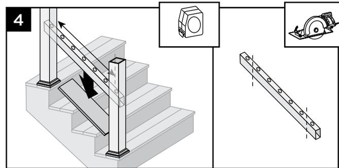
4. Set railing on top of deck board, making sure baluster holes are vertically aligned and mark line at each intersection. **When measuring, cut equal lengths from each side of railing allowing a minimum of 2" (51 mm) on each end from the last baluster hole to the end of the rail.** This will ensure proper baluster and bracket placement and equal spacing of balusters per each railing section.
