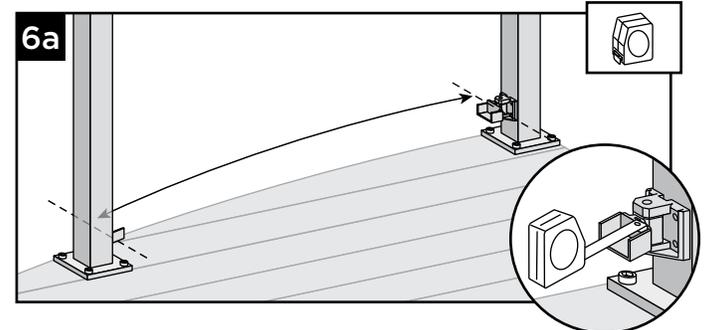
6a. With brackets in correct swivel location, measure distance from inside of bracket to inside of bracket. In addition, if tabbed bottom swivel brackets are installed the tab must be removed.
