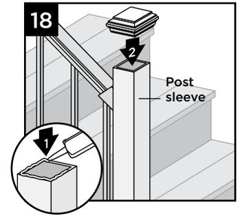
17. Attach post caps to Trex Signature posts (use of **rubber mallet** may be required for secure attachment).
