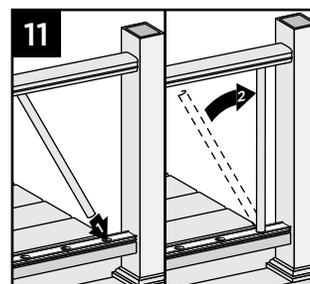
**Tip:** Ensure balusters are level prior to attempting to slide baluster spacer up. This will allow for the baluster spacer to move up freely and snap into upper rail. Use of a rubber mallet to gently tap balusters in level is recommended.
