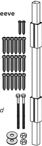
**\*NOTE:** If using 6x6 post sleeves, attach designated railing brackets using #8-15 x 1-3/4" (4.4cm) 316 stainless steel self-tapping screws (not provided). Pre-drilling IS REQUIRED when attaching brackets to designated posts. Use a 9/64" (3.6 mm) drill bit.
