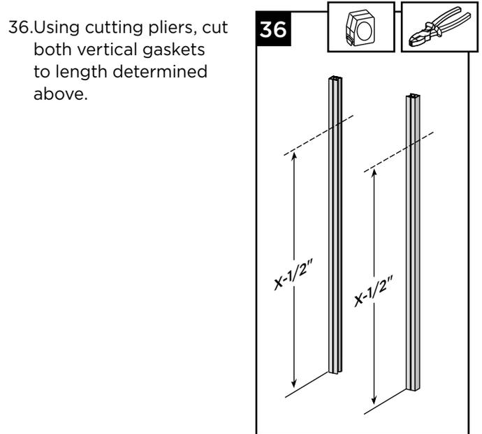
36. Using cutting pliers, cut both vertical gaskets to length determined above.
