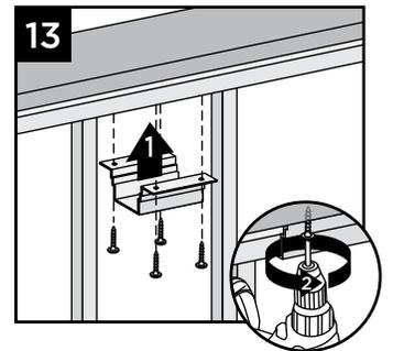
**NOTE:** Pre-drilling before attachment is recommended.
