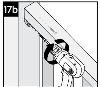
17b. Attach top stair rail bracket to lower post using two #8-10 x 3" screws (provided).
