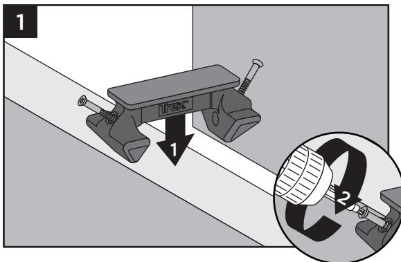
1. For butt joints, where boards meet over a single joist, install butt clip to shared joist as shown with 2 screws (supplied with clip).
