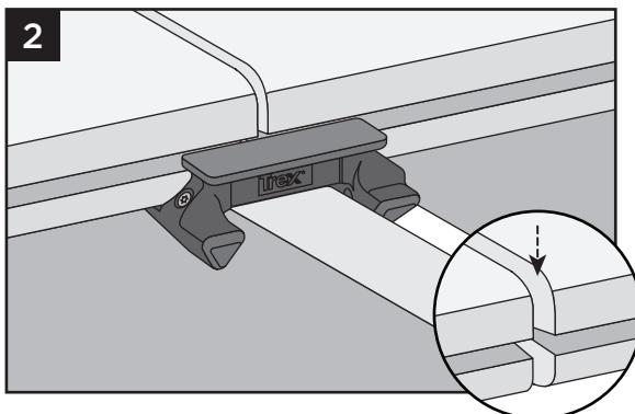
2. Properly gap decking per Trex requirements.
