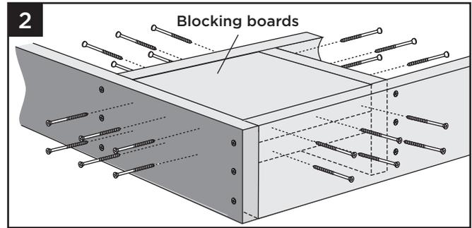
2. Install two 2" x 8" (51 mm x 203 mm) boards as blocking under post location. Securely attach blocking using a total of twenty-four 3" (76 mm) pressure-treated compatible screws (not provided).
