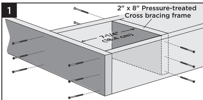
1. Install 2" x 8" (51 mm x 203 mm) cross bracing frame in between joists at 7-1/4" (184 mm). Attach a total of twelve 3" (76 mm) pressure-treated compatible screws (not provided).
