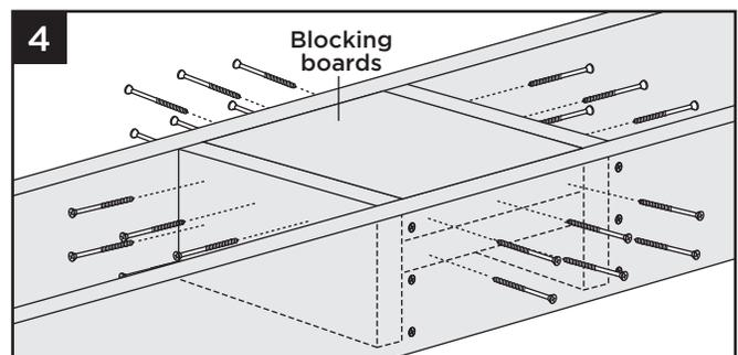
4. Install two 2" x 8" (51 mm x 203 mm) boards as blocking under post location. Securely attach blocking using a total of twenty-four 3" (76 mm) pressure-treated compatible screws (not provided).
