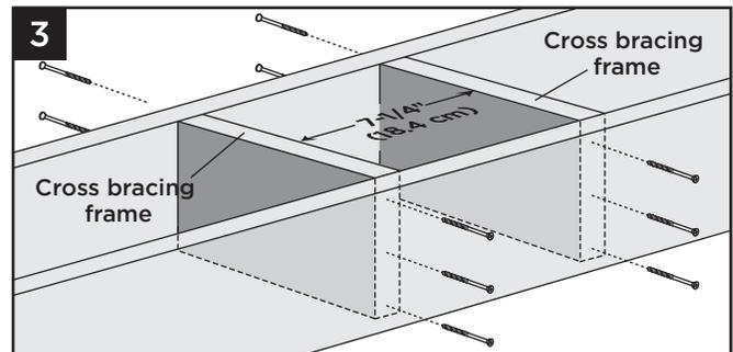
3. Install two 2" x 8" (51 mm x 203 mm) cross bracing frames in between joists at 7-1/4" (184 mm). Attach a total of twelve 3" (76 mm) pressure-treated compatible screws (not provided).
