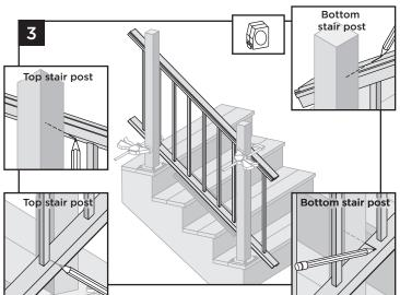
3. Mark stair rails to cut. At top stair post location, mark UNDERSIDE of lower and upper stair rails. At bottom stair post location, mark TOPSIDE of lower and upper stair rails.
