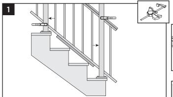
Use a 1" deck board as a spacer board and lay this on the stair treads between the posts. Place stair panel on top of the deck board and clamp stair panel to posts. Ensure that balusters are straight and positioned with equal spacing at post locations.
