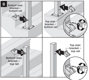
Center stair brackets on posts above the marked line and attach using two self-tapping screws (provided). In some cases it may be difficult to attach the stair bracket on the lower stair post. A 90° cordless drill is recommended to attach screws in this area.
