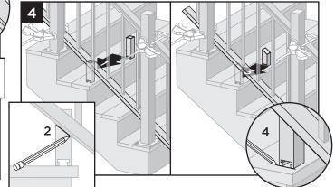
4. Mark location of angle on foot block and cut on mark. Then place foot block under the center of the bottom stair rail. Mark placement location of the base.
