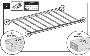
7. Remove panel and place on flat surface. Cut each end of the bottom and top stair rails 1/4" (0.6 cm) shorter than the mark on each end to allow for fit into stair rail brackets.
