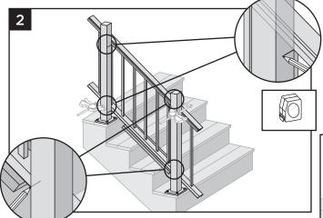
2. Mark posts for bracket locations. Mark at the underside of both top and bottom stair railing locations.
