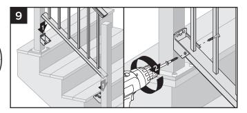
9. Attach stair panel to brackets using two self-tapping screws (provided) on each side of stair bracket.
