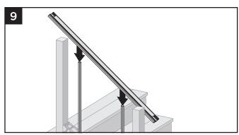
9. Position top stair rail onto balusters ensuring balusters are fully seated in top rail (position to side of post) and ENSURE that balusters are parallel with
