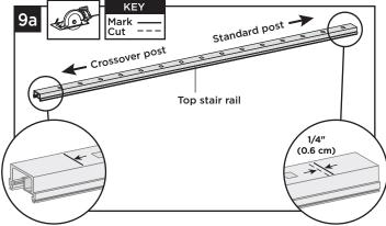
9a. Top stair rail along with rail insert must be cut differently on each side of the rail. Railing side that attaches to standard post should be cut 1/4" (0.6 cm) shorter than the mark to allow for fit into top rail bracket. Railing side that attaches to the crossover post should be cut directly on the mark to allow for fit into the crossover post bracket.
