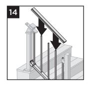
15a. For stair post-to-post configuration, attach top stair rail to top stair bracket (all types) using two self-tapping screws (provided) on each side of stair bracket.
