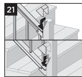
17. Attach "crowned" upper stair rail cover to upper stair rail by aligning cover on one side of rail. Then starting from one end of stair rail, snap cover onto opposing slot working down length of stair rail.
