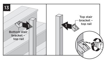
13. Remove upper stair rail and center upper stair fixed bracket on post **above** the marked line and attach using two self-tapping screws (*provided*).
