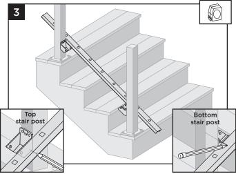
3 Position bottom stair rail along the nose of the stair treads. Ensure that before cutting, balusters holes are centered in between the posts and also allow for clearance for attachment to brackets. On top stair post location, mark UNDERSIDE of lower rail. On bottom stair post location mark TOPSIDE of lower rail at angled intersection of the bracket.
