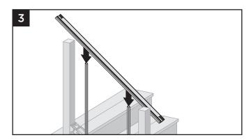
Position top stair rail onto balusters ensuring balusters are fully seated in top rail (position to side of post) and ENSURE that balusters are parallel with post. 4. Follow previous instructions marking and installation of either fixed or swivel bracket where this is required.
