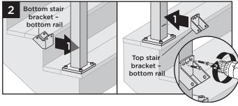
2. Center lower stair bracket on post above the marked line and attach using two self-tapping screws (provided). In some cases it may be difficult to attach the stair bracket on the lower stair post. A 90° cordless drill is recommended to attach screws in this area.
