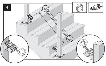
4. Cut each end of the bottom rail, rail insert, and bottom rail cover at the mark on each end to allow for fit into bottom stair rail brackets.
