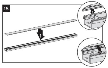
15. Attach "crowned" upper stair rail cover to upper stair rail by aligning cover on one side of rail. Then starting from one end of stair rail, snap cover onto opposing slot working down length of stair rail. GENTLE tapping with a rubber mallet may facilitate fastening.
