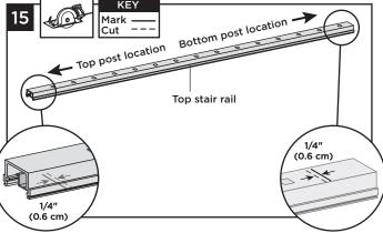
15. Cut each end of top stair rail along with rail insert 1/4" (0.6 cm) shorter than mark to allow for fit into top stair rail bracket.
