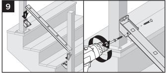
9. Set bottom stair rail into bottom stair rail brackets. Attach bottom stair rail to bottom stair bracket using two self-tapping screws (provided) on each side of bracket.
