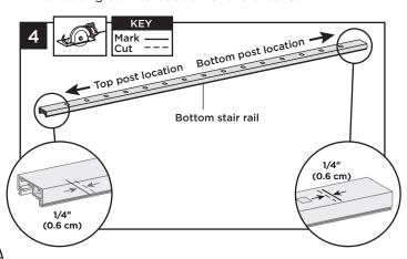
4. Cut each end of the bottom stair rail, rail insert, and bottom rail cover 1/4" (0.6 cm) shorter than the mark on each end to allow for fit into bottom stair rail brackets.
