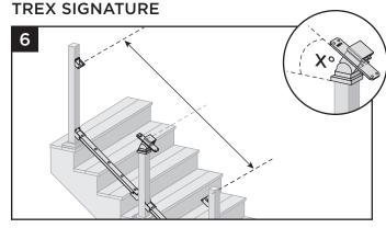
Determine location/height of the stair crossover swivel bracket by aligning the angle of this with the fixed brackets (or compound swivel brackets) already installed (posts can be cut if necessary).
