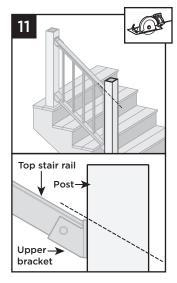
7a. Cut each end of top stair rail along with rail insert 1/4" (0.6 cm) shorter than mark to allow for fit into top stair rail bracket.
