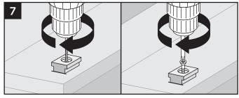
7. Place base (smaller side facing down) on decking surface. Pre-drill using a 3/16" bit. Attach base of foot block using one screw at an angle through base and into decking.
