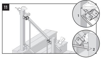
11. Mark a light line on posts at UNDERSIDE of where swivel bases (positioned correctly) meets the posts.
