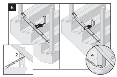
6. Temporarily set bottom rail in bottom brackets, and place foot block towards the nose of the stair tread along the side of the bottom rail. Mark location of angle on foot block and cut on mark. Then place foot block under the center of the bottom rail. Mark placement location of the base. Remove lower rail.
