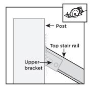
12. Place deck boards over top rails. PLACE DECK BOARD ON TOP RAIL TO CHECK FOR PROPER FIT AND RAIL CLEARANCE AT BRACKET LOCATIONS. **DECK BOARD MAY** REQUIRE EITHER A NOTCH CUT ON THE UNDERSIDE OR SLIGHT PLANING ON THE
