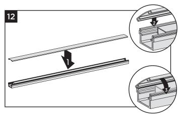
12. Attach "crowned" upper stair rail cover to upper stair rail by aligning cover on one side of rail. Then, starting from one end of stair rail, snap cover onto opposing slot working down length of stair rail.
