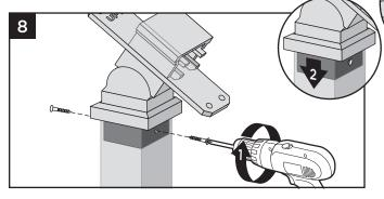
8. Attach stair crossover swivel bracket to post with two self-tapping screws (*provided*). Slide cover over post to hide screws.
