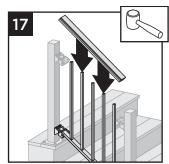
16. Place balusters into holes in lower stair rail by snapping fully into place. In some cases, **GENTLE** tapping with a **rubber mallet** may facilitate fastening.
