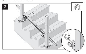
3. With brackets in correct swivel locations, measure distance from inside of swivel bracket to inside of swivel bracket. Ensure that before cutting, balusters holes are parallel and centered in between the posts and also allow for clearance for attachment to brackets. Mark bottom stair rail at each intersection.
