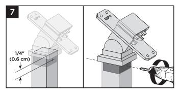
7. Once location/height is determined, center and predrill two holes (using a drill bit slightly smaller than that of self-tapping screw diameter) on opposite sides of post, approx. 1/4" (0.6 cm) from top of post. Drill through the post and into the stair crossover swivel bracket on each side.
