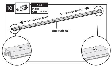
10. Cut each end of the top stair rail along with rail insert on the mark line to allow for fit into the crossover post bracket on each side.
