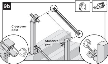
9b. When going from standard stair post to stair crossover post, measurement must be taken from inside of top horizontal stair swivel bracket to inside lip of stair crossover bracket. Crossover post will need to be modified to have swivel crossover bracket installed.
