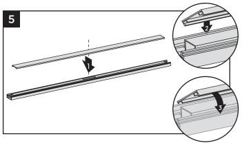
5. Attach "flat" bottom stair rail cover to bottom stair rail. Align cover on one side of the bottom rail in slot on side of rail. Then starting from one end of rail snap cover onto opposing slot working down the length of the rail. In some cases, **GENTLE** tapping with a **rubber mallet** may facilitate fastening.
