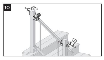
10. Clamp brackets to side of rail with brackets in correct swivel location/angle (this is important to ensure correct location of swivel brackets).
