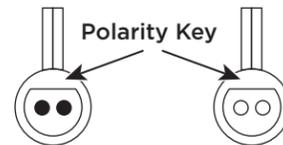
3. Plug the power supply into a GFCI-protected wall socket. If you see the red "FAULT" light, your system has reversed polarity. Check the polarity key on your input cable and correct any problems before proceeding.
