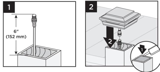
1. Connect male lead from wiring to female connector from cap. Also attach male-to-male connection wires in between each splitter. Continue until all wiring from lights is attached to splitters and connector wires are attached in between splitters. (See Making Connections section for details.)
