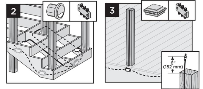
2. Wiring can be run under deck and behind risers. Staple to frame with cable staples at least 1/4" (6 mm) wide. **DO NOT** crush wire insulation with staples.
