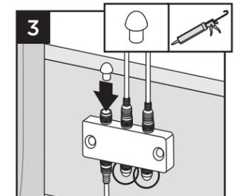
2. Attach male lead from lights to female connections on splitter. Also attach male-to-male connection wires in between each splitter. Continue until all wiring from lights are attached to splitters and connector wires are attached in between splitters.
