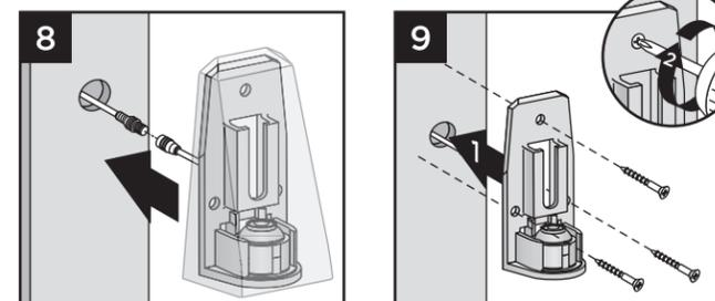
8. Connect male connector to female connector on light housing.
