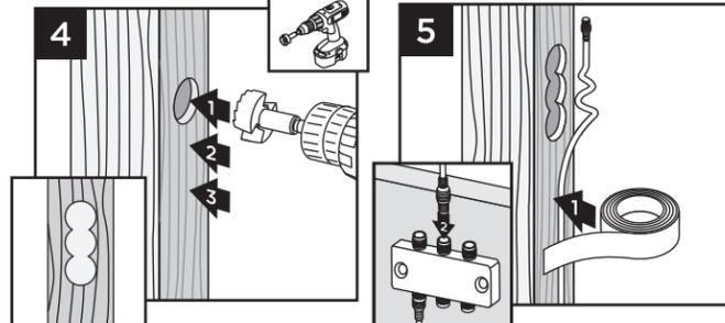
4. Drill out existing hole on pressure-treated post 3/4" (19 mm) deep. Drill two additional holes vertically below main hole—this will allow space for wiring after post sleeve is attached.
