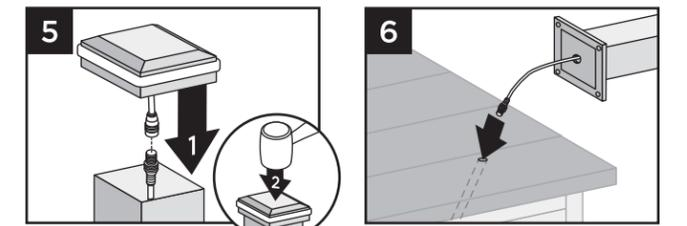
5. Connect the female connector on the post cap light to this wire and, using a rubber mallet, gently tap the cap onto top of post until it is secure.
