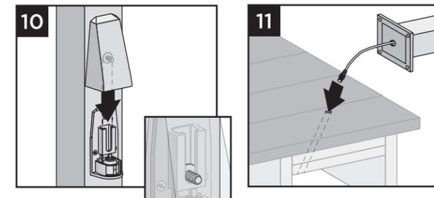
10. Slide light cover down over backing plate, adjusting mounting screws as necessary to achieve a tight fit.
