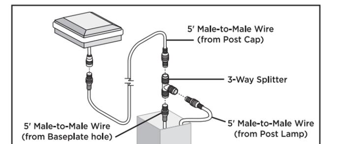
**NOTE:** If connecting a Trex Wedge Deck Rail Light as well, a 3-way adapter and extra 5' male-to-male wire (not provided) can be used inside the post so that only one wire must be run through the hole in the base of the post (and post blocking). This is optional.
