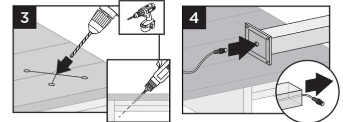
3. Using a 9/16" (14 mm) x 6" (152 mm [or longer]) drill bit, drill a diagonal hole through the decking and blocking. Ensure that the angle will allow wire to not be pinched by support plate under blocking (if using Trex ALPOSTHWDECK mounting kit). (See *Making Connections* section for details.)
