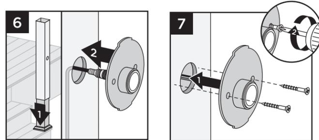
6. Slide post sleeve back over post. If using a post sleeve skirt, make sure to install the skirt first. Connect plug on deck rail light to lead wire and tuck wiring into previously drilled-out pockets on post.
