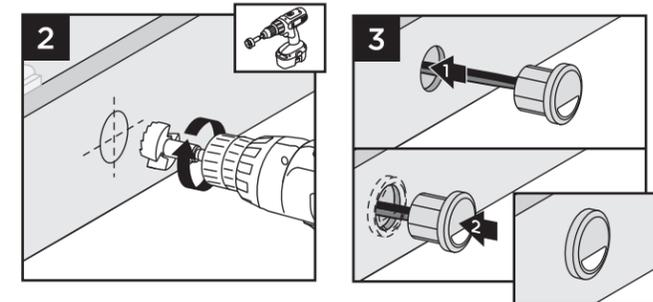
2. Drill a 1" (25 mm) diameter hole at least 1" (25 mm) deep into riser. If riser material is thicker than 1" (25 mm), use a 1/2" (13 mm) drill bit to create a passage for wires.
