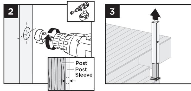
2. Drill a 1" (25 mm) hole through post sleeve. Drill deep enough to mark location on pressure-treated post.
