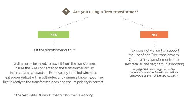
If the Transformer is working but all lights are out, the connection of the 20' transformer wire is the problem, or the wiring is not connected correctly with wire nuts. For Trex LightHub® plug-and-play lighting, ensure that the female splitter pins are intact (and not bent). If the lights still don't work, try another port.
