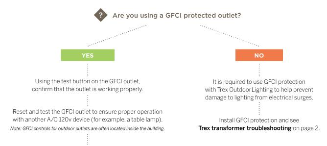
If the GFCI outlet is working, but the lights are not working, see **Trex timer troubleshooting** on page 2.
