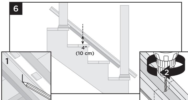
6. Mark approximate location for foot block, allowing a measurement of 4" maximum. Invert the bottom rail, and at marked location drill a hole using a 3/16" drill bit in the center of the channel. Foot block is to be installed at last step. For spans over 6' in commercial applications, mark and drill two locations spaced evenly apart for two foot blocks.
