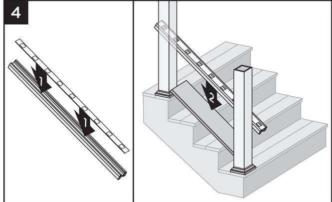
stair rail on top of the deckboard
