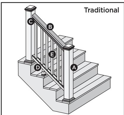
Cutting post sleeves is **NOT** required. Ensure both top and bottom post/post sleeves are tall enough to accommodate top rail and 2 x 4.
