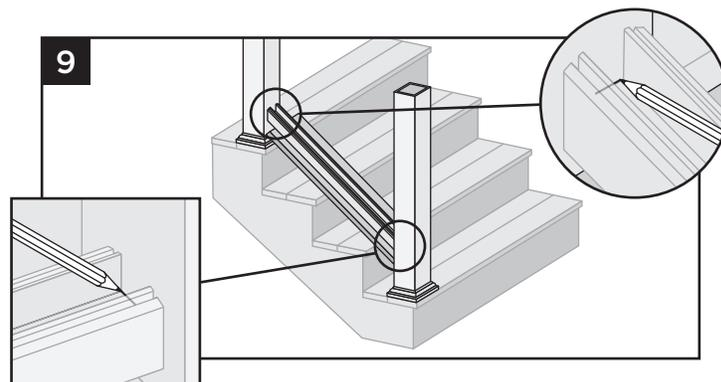
9. Mark both posts on inside channel of the bottom stair rail. Remove bottom stair rail.
