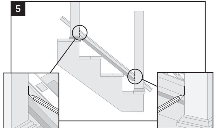
5. Use the lower and upper stair post to set the length of the bottom stair rail. Ensure that baluster spacer holes are spaced evenly between posts. Also allow for a minimum of 1-1/2" (292 mm) at each end of the stair rail for bracket placement and baluster clearance. Mark rail at post intersections.
