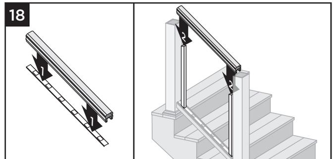
18. Remove baluster spacer from top stair rail and place rail in between posts on top of balusters, **ENSURING** that balusters remain parallel to post.
