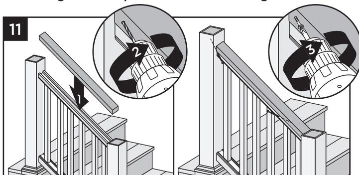
11. Pre-drill a pilot hole and toenail 2-1/2" (6.4 cm) composite deck screw at each end of 2 x 4 into post on back side of stair rail (side not facing decking).
