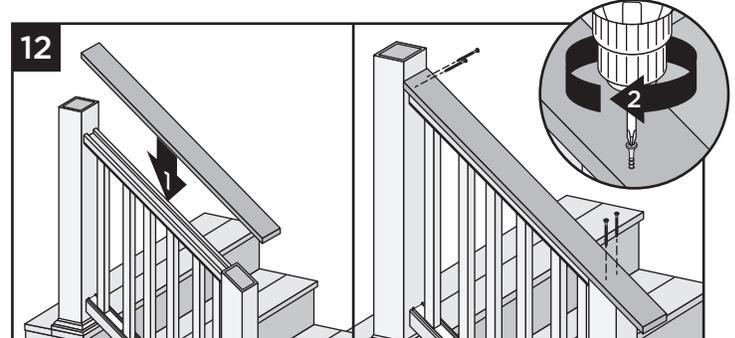
12. Place deck board on top rail and attach board to posts using two Trex recommended composite decking screws (use two screws per each post).
