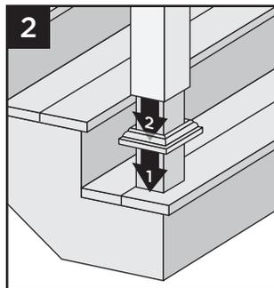
**NOTE:** Shims can be used to plumb post sleeves.
