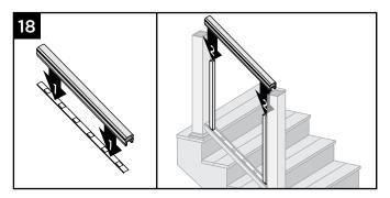
Remove baluster spacer from top stair rail and place rail in between posts on top of balusters, ENSURING that balusters remain parallel to post.
