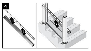
4. Snap baluster spacer into bottom stair rail and lay bottom stair rail on top of the deckboard
