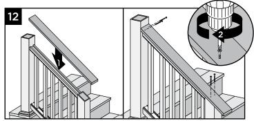
12. Place deck board on top rail and attach board to posts using two Trex recommended composite decking screws (use two screws per each post).
