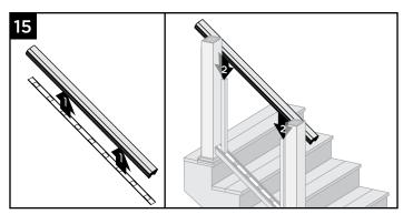
15. Snap baluster spacer into top stair rail. Position top stair rail onto balusters, ensuring balusters are fully seated in rail (position to side of post), and **ENSURE** that balusters are spaced evenly **AND** parallel with post. Also allow for a minimum of 1-1/2" (292 mm) at each end of the stair rail for bracket placement and baluster clearance.
