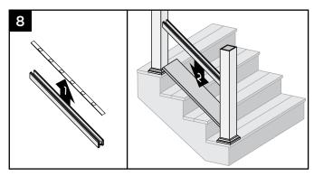
8. Remove baluster spacer from bottom rail and place rail in between posts, keeping rail on deckboard.
