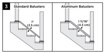
3. If using standard balusters, place a 1" deckboard on the nose of the stair tread. If using aluminum balusters, use a scrap piece of wood measuring at least 1-11/16" thick, and place on the nose of the stair tread.
