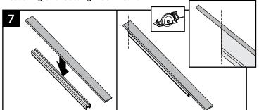
7. Using the cut top rail as template, cut deck board at upper post location at same angle as the top rail. Leave a generous amount of deck board material at lower post location as this will allow for overhang and can be cut later.
