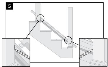
Use the lower and upper stair post to set the length of the bottom stair rail. Ensure that baluster spacer holes are spaced evenly between posts. Also allow for a minimum of 1-1/2" (292 mm) at each end of the stair rail for bracket placement and baluster clearance. Mark rail at post intersections.
