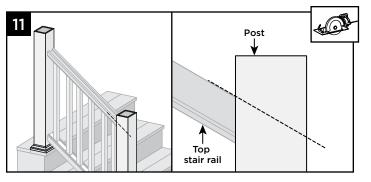
11. Cut post and post sleeves to proper angle so cut is flush with the top rail. Be careful to not cut top rail.
