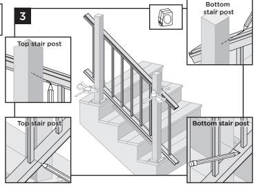
Mark stair rails to cut. At top stair post location, mark UNDERSIDE of lower and upper stair rails. At bottom stair post location, mark TOPSIDE of lower and upper stair rails.
