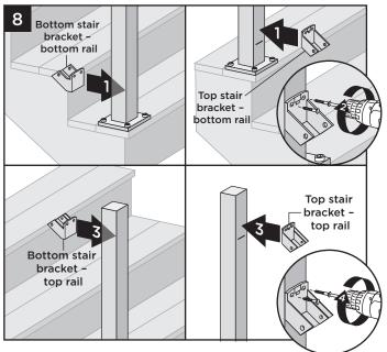
8. Center stair brackets on posts above the marked line and attach using two self-tapping screws (provided). In some cases it may be difficult to attach the stair bracket on the lower stair post. A 90° cordless drill is recommended to attach screws in this area.
