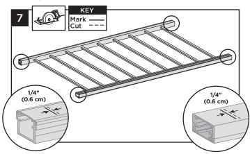
7. Remove panel and place on flat surface. Cut each end of the bottom and top stair rails 1/4" (0.6 cm) shorter than the mark on each end to allow for fit into stair rail brackets.
