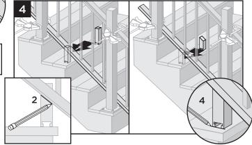
4. Mark location of angle on foot block and cut on mark. Then place foot block under the center of the bottom stair rail. Mark placement location of the base.
