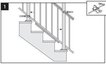
Use a 1" deck board as a spacer board and lay this on the stair treads between the posts. Place stair panel on top of the deck board and clamp stair panel to posts. Ensure that balusters are straight and positioned with equal spacing at post locations.
