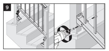
9. Attach stair panel to brackets using two self-tapping screws (provided) on each side of stair bracket.
