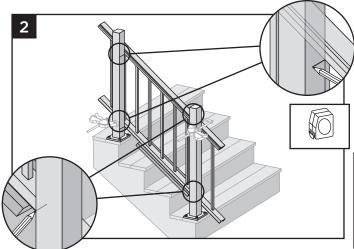
Mark posts for bracket locations. Mark at the underside of both top and bottom stair railing locations.
