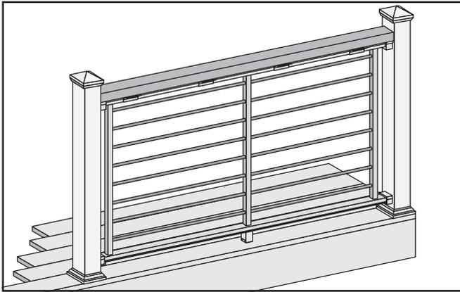
**Important:** Only use with Pressure-treated post, Trex Post Mounts or Trex Joist Mount Post WITH Trex post sleeves. Trex Signature Posts and Joist Mount Posts cannot be used with Rod Rail Traditional.
