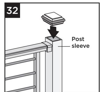
32. Secure post caps with silicone or PVC adhesive. (apply adhesive on the inside self-centering/corner tabs).
