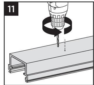
**NOTE:** Clean any burrs from edges of holes to ensure good fit on both sides.
