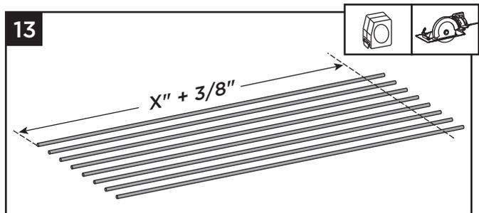
13. Cut rods to the length measured in previous step.
