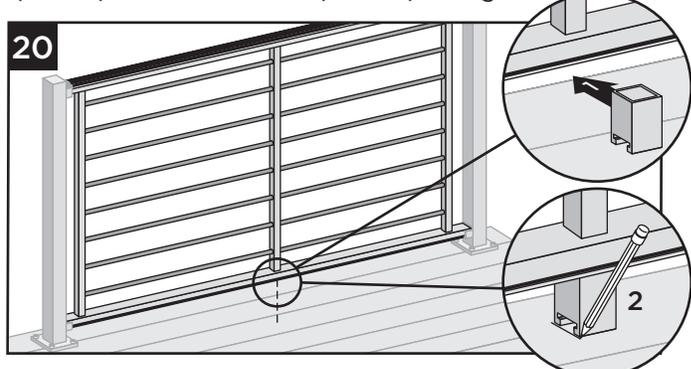
20. Temporarily drop rod rail panel into brackets. To ensure correct location, place foot block under center of bottom panel. Mark to provide placement location of base. Once marked remove panel.
