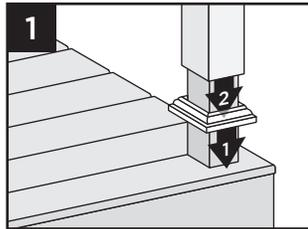
**NOTE:** Shims can be used to plumb post sleeves.
