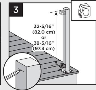
2. Center lower bracket on post **above** the marked line and attach using four self-tapping screws (*provided*).
