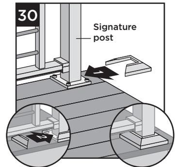
30. Attach provided post skirt to bottom of posts when using Trex Signature posts.
