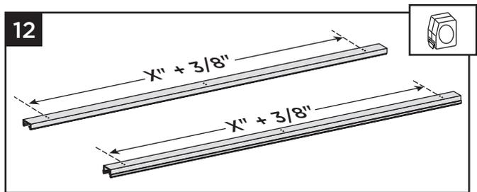
12. Measure the distance between the end (outer) holes (X") on top or bottom rail and add 3/8" to this measurement.
