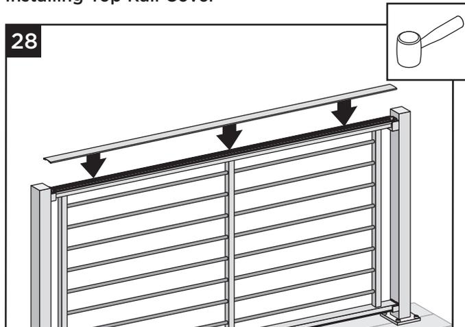
28. Using a mallet, install top rail cover.
