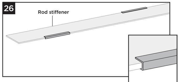
26. Attach tape (qty 6 provided) to alternating sides of the rod stiffener as shown.
