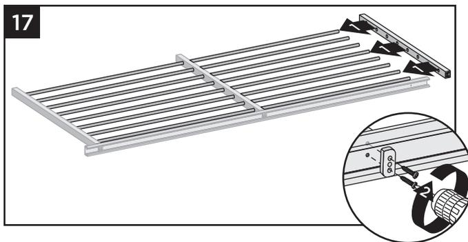
17. Slide end vertical onto rods and attach to bottom rail using HZ spacer and screws provided. HZ spacer should be oriented so the ribbed side of the spacer is not showing.
