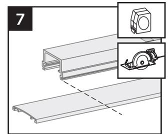
7. Mark and cut top rail cover same length as top rail for all top rail configurations.
