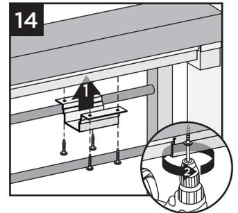
**NOTE:** Pre-drilling before attachment is recommended.
