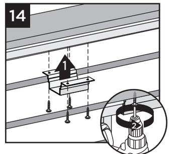
**NOTE:** Pre-drilling before attachment is recommended.
