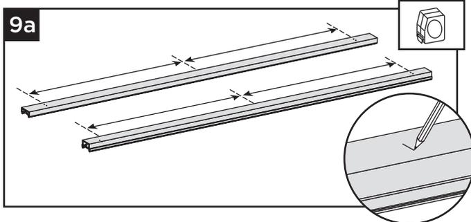
9a. Measure the distance between the vertical end holes on **both top and bottom rails**. Mark the center.
