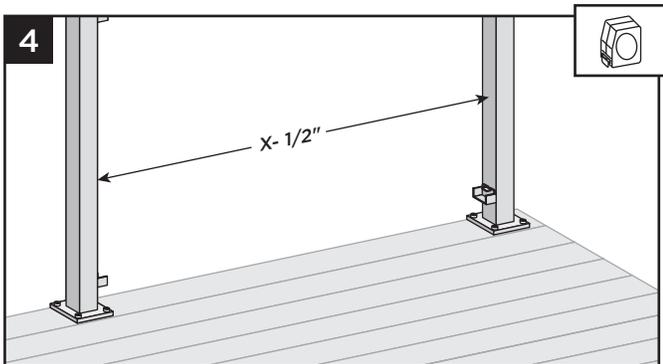
4. Measure distance between posts (X), and subtract 1/2" for bracket clearance.
