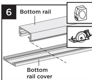
6. Mark and cut bottom rail cover the same length as bottom rail.
