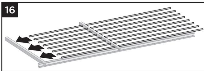
16. Slide all rods through intermediate supports and into end vertical support.
