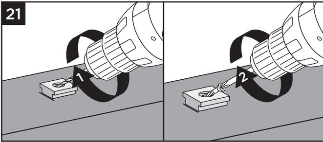
21. Place base (smaller side facing down) on decking surface. Pre-drill using a 3/16" bit. Attach base of foot block using one screw at an angle through base and into decking.
