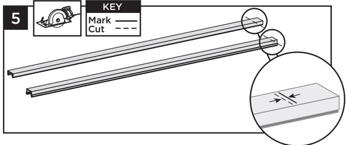
5. Cut both bottom and top rail to length as determined above.
