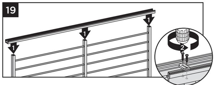
19. Install top rail to all vertical and end supports using HZ spacer and screws provided. HZ spacer should be oriented so the ribbed side of the spacer is not showing.
