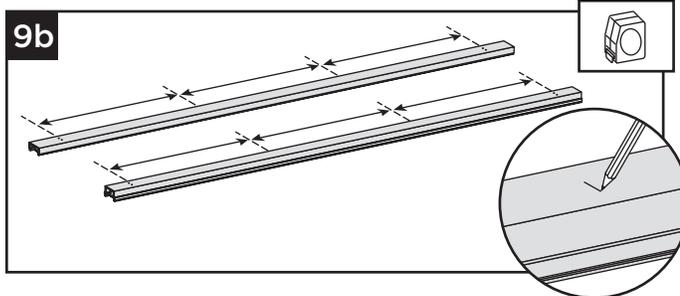
9b. Measure the distance between the vertical end holes on **both top and bottom rails**. Divide the distance into thirds and make two marks on top and bottom rails.
