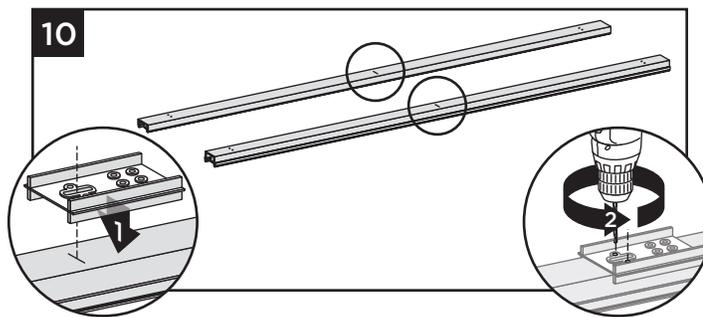
10. Using the slot on the HZ template, locate marked line and drill two 7/64" pilot holes (or mark with a punch).
