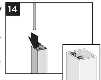
**NOTE:** There are two anti-rattle strips for each support which can only be inserted in one side.
