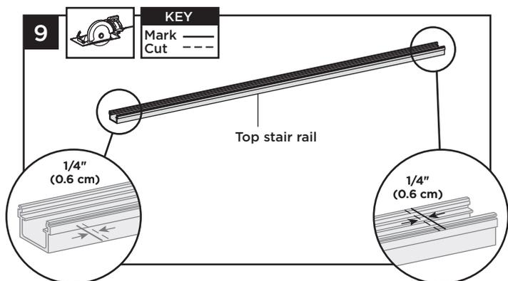
9. Cut each end of top stair rail and top rail cover  $1/4"$  (0.6 cm) shorter than mark to allow for fit into top stair rail bracket.
