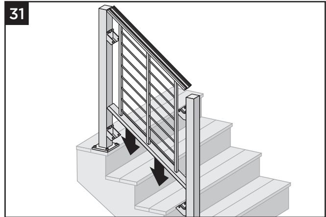
31. Drop assembled stair rod rail panel into brackets.
