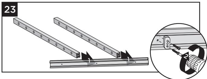
23. Install lowest end vertical and all intermediate verticals to bottom rail using ST Wedge Spacer and screws provided.
