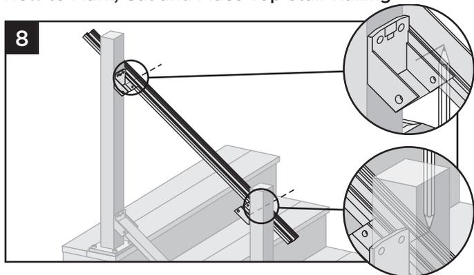
8. Position top rail to side of post. Mark top stair rail at each location stated. On **UPPER STAIR POST**, mark from underside of bottom rail. On **LOWER STAIR POST**, mark from topside of bottom rail.
