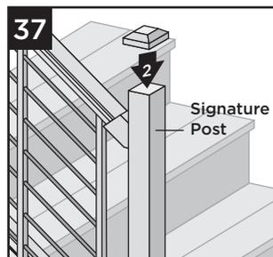
37. Attach post caps to Trex Signature posts. (Use of **rubber mallet** may be required for secure attachment.)
