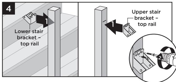
4. Center upper stair brackets on posts **below** the marked lines and attach using two self-tapping screws (*provided*).
