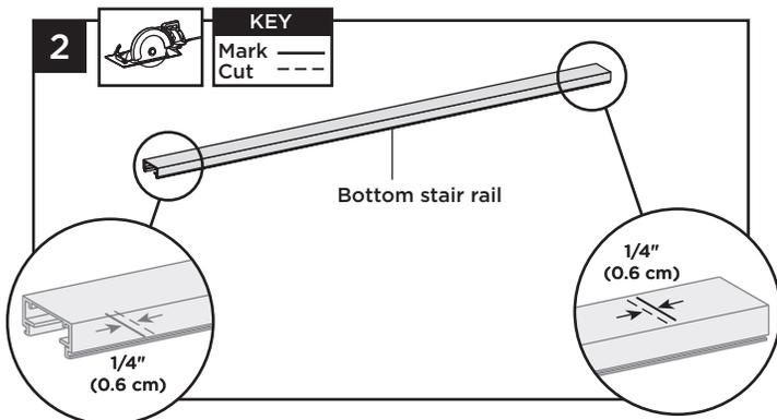
2. Cut each end of the bottom stair rail and bottom rail cover 1/4" (0.6 cm) shorter than the mark on each end to allow for fit into bottom stair rail brackets.
