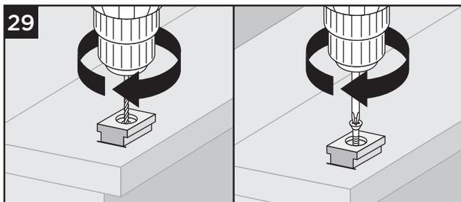
29. Place base (smaller side facing down) on decking surface. Pre-drill using a 3/16" bit. Attach base of foot block using one screw at an angle through base and into decking.
