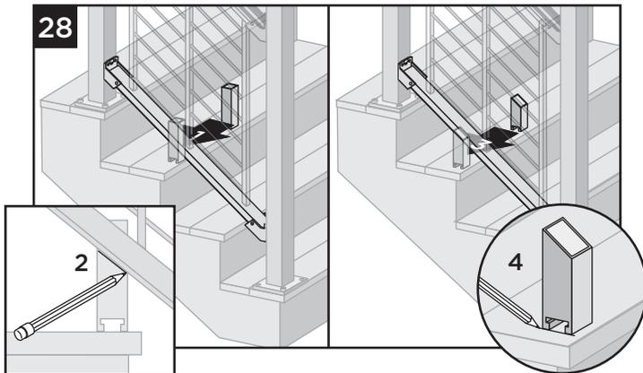
28. Temporarily drop assembled stair rod rail panel into brackets. To ensure proper location place foot block towards the nose of the stair tread along the side of the bottom rail. Mark location of angle on foot block and cut on mark. Then place foot block under the center of the bottom rail. Mark placement location of the base.
