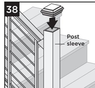
38. Secure post caps with silicone or PVC adhesive (apply adhesive on the inside self-centering/corner tabs).
