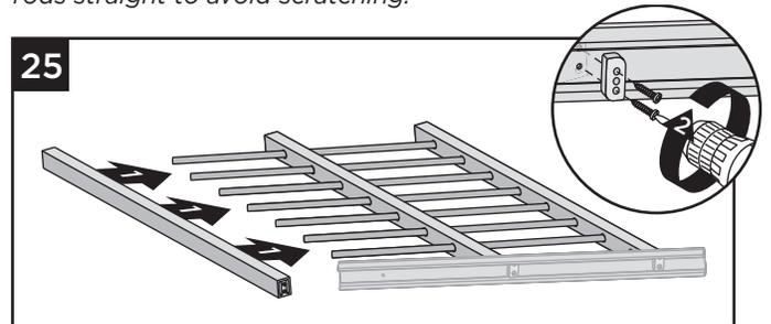
25. Slide upper end vertical onto rods and attach to bottom rail using ST Wedge Spacer and screws provided.
