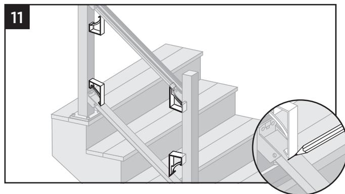
11. Using the long edge of the stair template, mark the location of the end verticals on the upper and lower rails.
