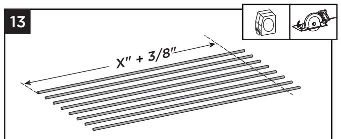
13. Cut rods to the length measured in previous step.
