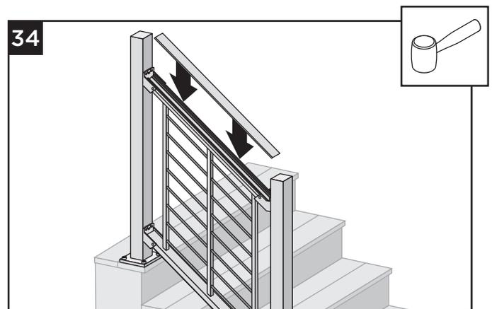
34. Using a mallet, install top rail cover.
