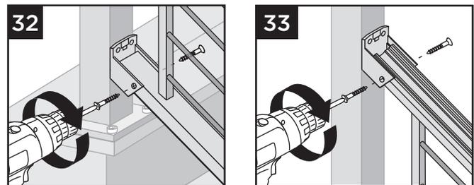
32. Attach bottom stair rail to bottom stair bracket using two self-tapping screws (*provided*) on each side of bracket.
