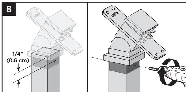
8. Once location/height is determined, center and predrill two holes (using a drill bit slightly smaller than that of self-tapping screw diameter) on opposite sides of post, approximately 1/4" (0.6 cm) from top of post. Drill through the post and into the stair crossover swivel bracket on each side.
