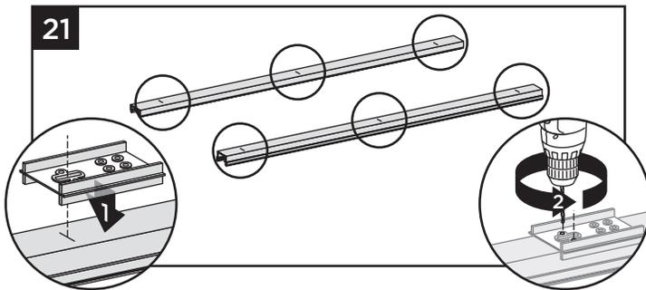
21. Using the slot on the HZ template, locate marked line and drill two 7/64" pilot holes at each mark (or mark with a punch).
