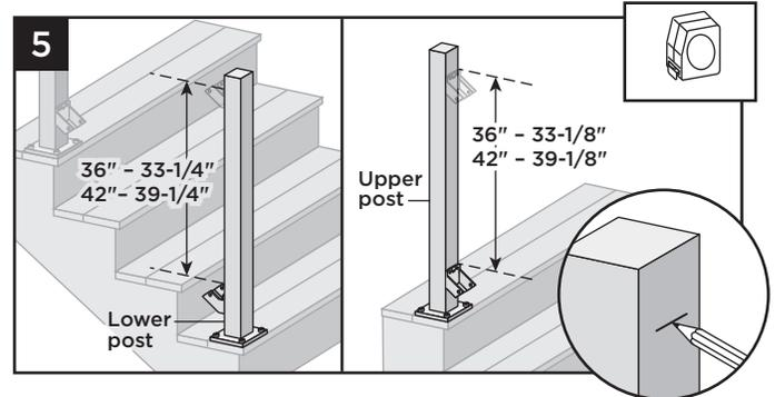
5. **On Lower Post** – From top of lower bracket, measure up and mark with light line (33-1/4" for 36" rail; 39-1/4" for 42" rail).
