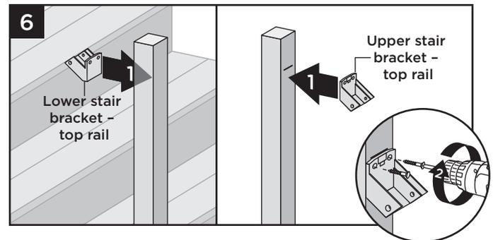
6. Center upper stair brackets on posts **below** the marked lines and attach using two self-tapping screws (provided).
