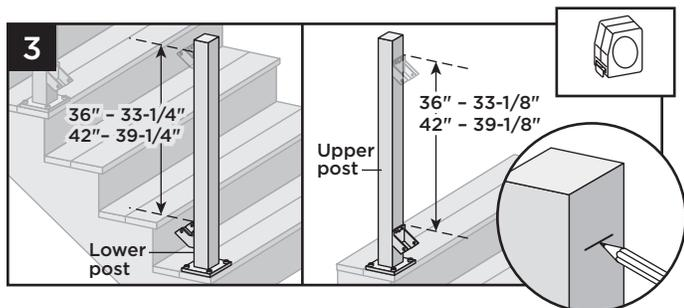
3. **On Lower Post** - From top of lower bracket, measure up and mark with light line (33-1/4" for 36" rail; 39-1/4" for 42" rail).
