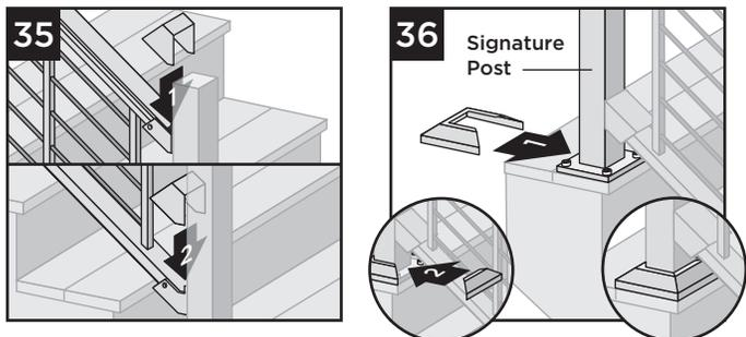
35. Attach corresponding bracket covers over opening in upper and bottom rails.
