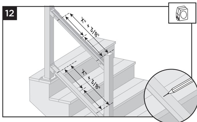
12. Measure and mark the mid-line (6' sections) of the two end marks of the top and bottom rail. Take that measurement and add  $3/8"$  for rod length in next step.
