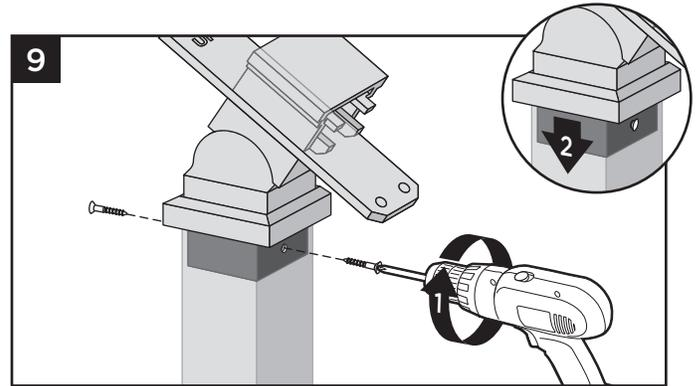
9. Attach stair crossover swivel bracket to post with two self-tapping screws (provided). Slide cover over post to hide screws.
