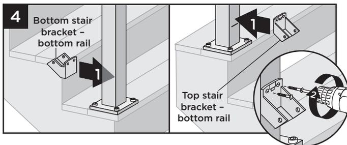
4. Center lower stair bracket on post above the marked line and attach using two self-tapping screws (provided). In some cases it may be difficult to attach the stair bracket on the lower stair post. Recommend using a 90° drill adapter or loosen the post to get access to the lower bracket screw holes.
