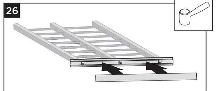
26. Using a mallet, install bottom rail cover onto bottom rail.
