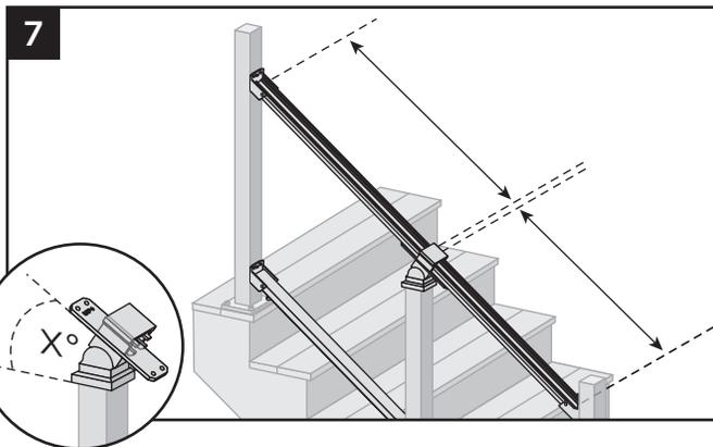
7. Determine location/height of the stair crossover swivel bracket by aligning the angle of this with the fixed brackets already installed. Note that the crossover post may need to be cut to ensure the top stair rail is parallel to the bottom stair rail.
