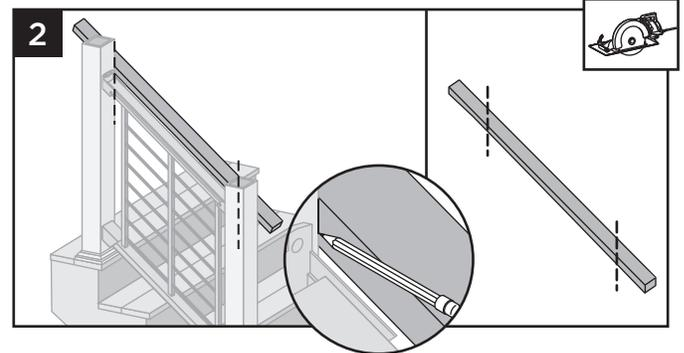
2. Place 2 x 4 beside top rail. Mark and cut (both ends need to be cut on an angle for proper fit).
