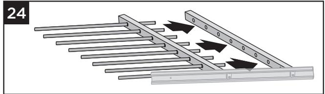
24. Slide rods into lower end and all intermediate verticals.
