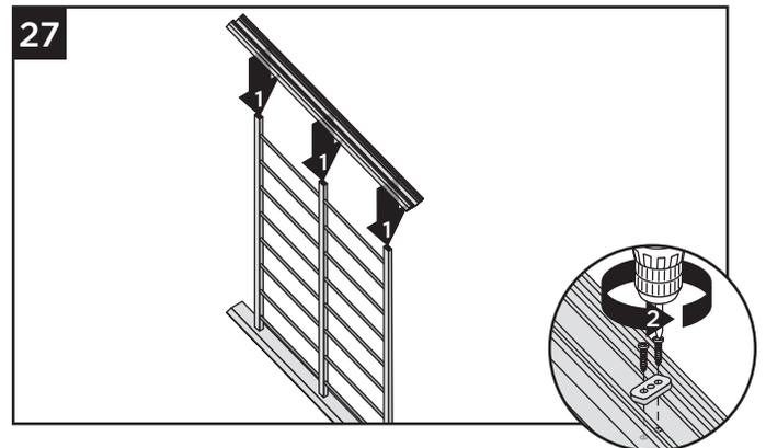
27. Install top rail to all vertical and end supports using S Wedge Spacer and screws provided.
