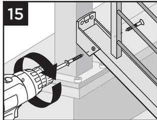
16. For stair crossover post configuration, fasten upper stair rail to swivel crossover post bracket by installing screws diagonally through crossover stair bracket into upper rail using two self-tapping screws (provided) on each side.
