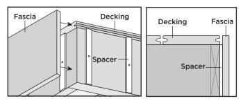
Install 3/16" to 1/4" thick x minimum 1" wide exterior grade spacers (these should be cut the same length as the rim joist), and spaced 9" on center. Install fascia screws as stated below at spacer locations (ensure that spacer screw does not interfere with fascia screw).
