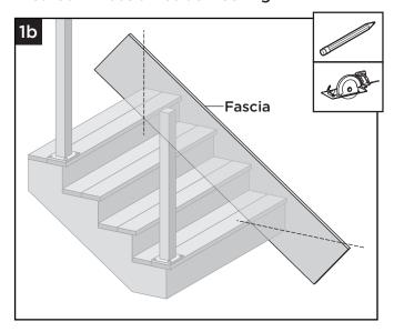
1b. Another option is cutting fascia plumb to the rim joist at the top and flush at the bottom of the stairs as shown.
