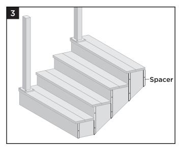
3. Spacers should be installed like that of standard decking, ensuring these are spaced 9" apart (see previous page for detailed information on all requirements for spacers)
