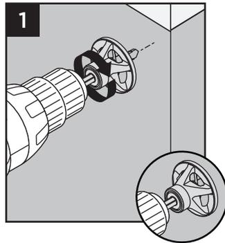
**NOTE:** This teal counterbore tool and teal Enhance/Fascia HEXSTIX® depth setter can also be used with Trex Enhance Deck Plug installations
