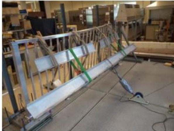
Photo No. 2 Uniform Test Load at 45°
