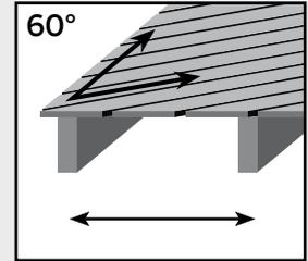
At a 60° angle, maximum joist spanning is 51 mm less than listed in the chart below.
