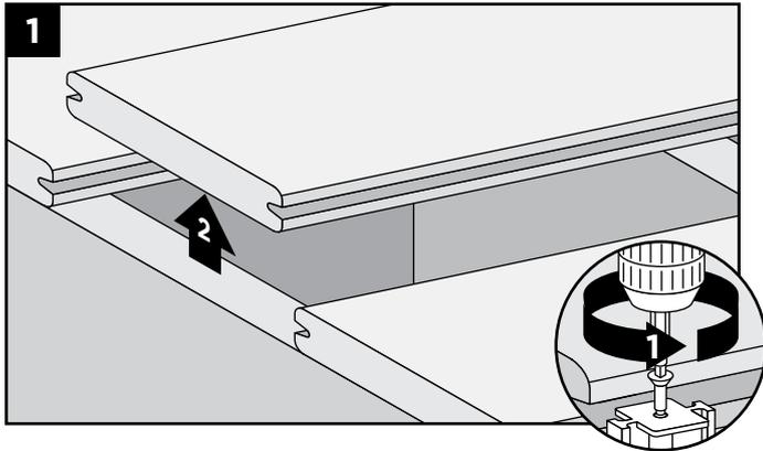
1. Remove screws from fasteners on both sides of board to be replaced and remove board.
