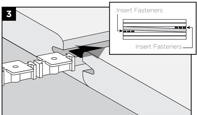
3. Slide a fastener for each joist into board grooves from both ends of the board.
