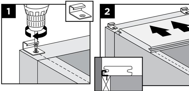
1. Install start clips on edge of ledger board, centered on each joist. Secure clips with screws.
