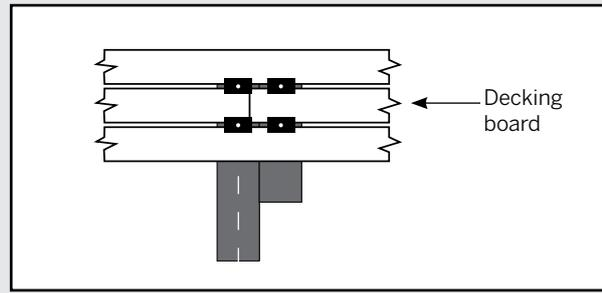
1. Install 254 mm - 305 mm framing boards along joists where seams will butt.
