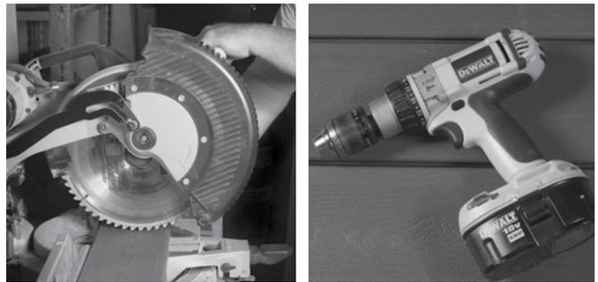
When using a miter saw, we recommend a 254 mm - 305 mm saw blade with 40 teeth or less.
