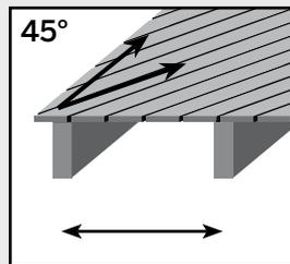
At a 45° angle, maximum joist spanning is 102 mm less than listed in the chart below.
