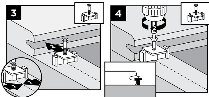
3. Insert fastener into grooved edge of deck board.
