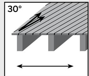
At a 30° angle, maximum joist spanning is 1/2 of the distance listed in the chart below.
