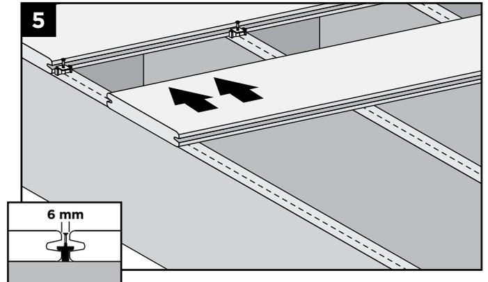
5. Slide second board into place, making sure fasteners fit into groove. Install the next universal fastener on the other side of the second board in the same manner as Steps 3 and 4. **DO NOT** fully tighten the screw.
