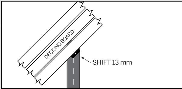
**ALWAYS start in corner** with a small triangular piece of decking at 45° and work outwards. Install Trex Hideaway fasteners 13 mm off center to keep fastener screws in middle of joists.
