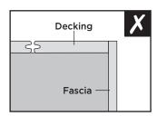
Do Not install fascia in the method shown here. The fascia board must be attached fully to the rim joist and cannot run parallel to the decking surface.
