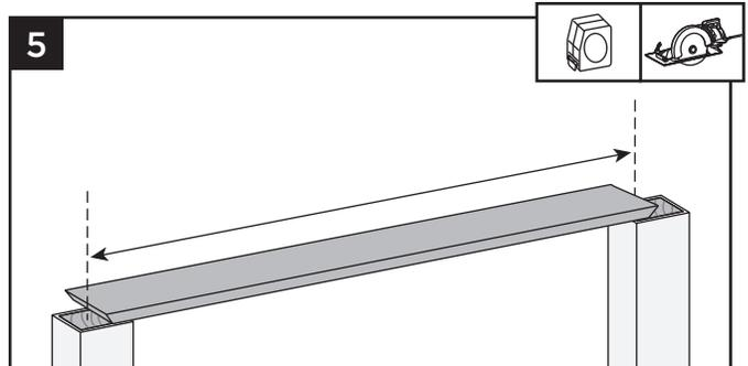
5. Cut deck boards to appropriate length of railing span, remembering to include extra space on each side of the deck board to allow for attachment to the post. Decking boards must cover 1/2 of the pressure-treated post to allow this to be fastened later.
