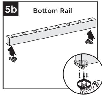
**NOTE:** For ease of bracket attachment place rail against stationary flat vertical surface along with bracket.
