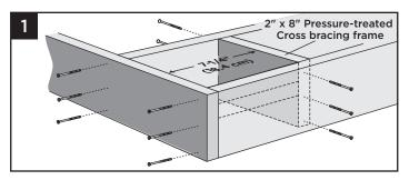
1. Install 2" x 8" (5.1 cm x 20.3 cm) cross bracing frame in between joists at 7-1/4" (18.4 cm). Attach a total of twelve 3" (7.6 cm) pressure-treated compatible screws (not provided).
