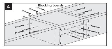
4. Install two 2" x 8" (5.1 cm x 20.3 cm) boards as blocking under post location. Securely attach blocking using a total of twenty-four 3" (7.6 cm) pressure-treated compatible screws (*not provided*).
