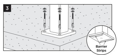
3. Insert the (2) stainless steel barrier strips under the mounting bolt holes. Use appropriate shims if posts are not plumb. Secure post mount with the four expansion anchors, washers and nuts.
