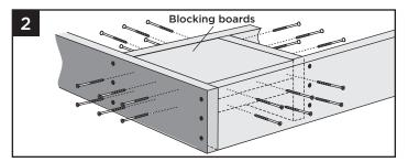
2. Install two 2" x 8" (5.1 cm x 20.3 cm) boards as blocking under post location. Securely attach blocking using a total of twenty-four 3" (7.6 cm) pressure-treated compatible screws (not provided).
