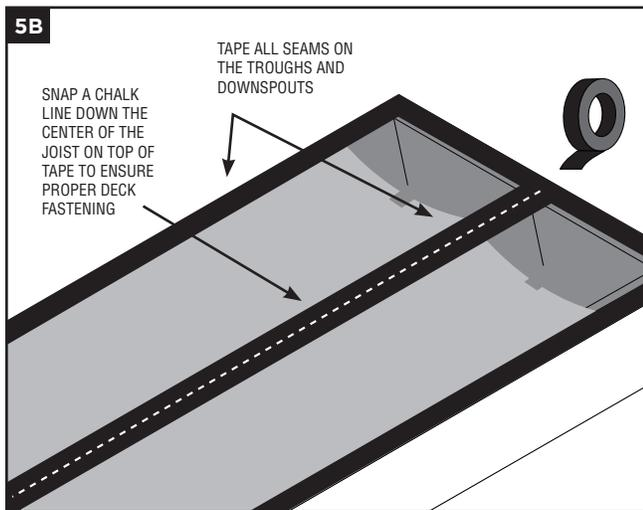
**NOTE:** *The butyl tape should never be put directly on the board without the trough material or a downspout below it.*
