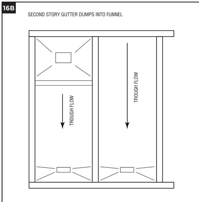
»Place downspout in rectangle (do not remove openings).
